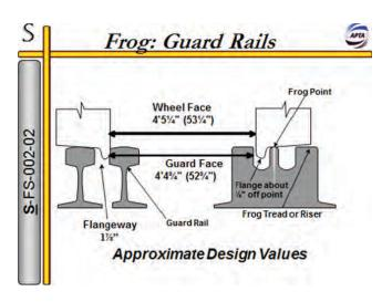
Item 32—Guard check gage: This is a measurement from the gage face of the frog to the guard face of the opposing guardrail. This is a minimum measurement. If this measurement is less than the criteria, then there is an opportunity for the wheel operating over the frog to hit the point of the frog or traverse in the wrong direction, causing a derailment.
