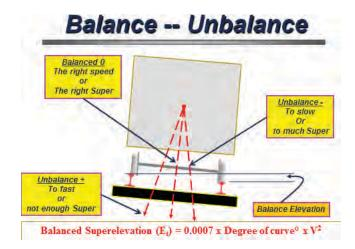
FIGURE 3 Balance-unbalance.
