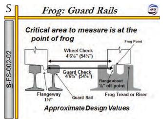
Item 27—Restraining rail flangeway: This is the minimum distance between the gage face of the running rail and the back side of the restraining rail (guard rail).
