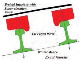
FIGURE 2 Typical interface with super-elevation: dynamic.
