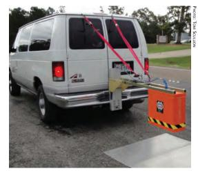
SHRP 2 research has explored highway preservation systems such as air-coupled ground-penetrating radar.
