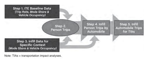
Figure 2.1. Approach for estimating vehicle trip generation.
