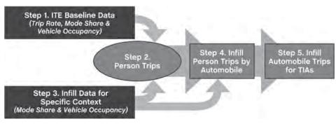
Diagram representing the approach for estimating vehicle trip generation for infill development based on adjusting ITE baseline trip generation data. The infill data used in the process can be derived from the methods described in this chapter. Note: TIAs = transportation impact analyses.
