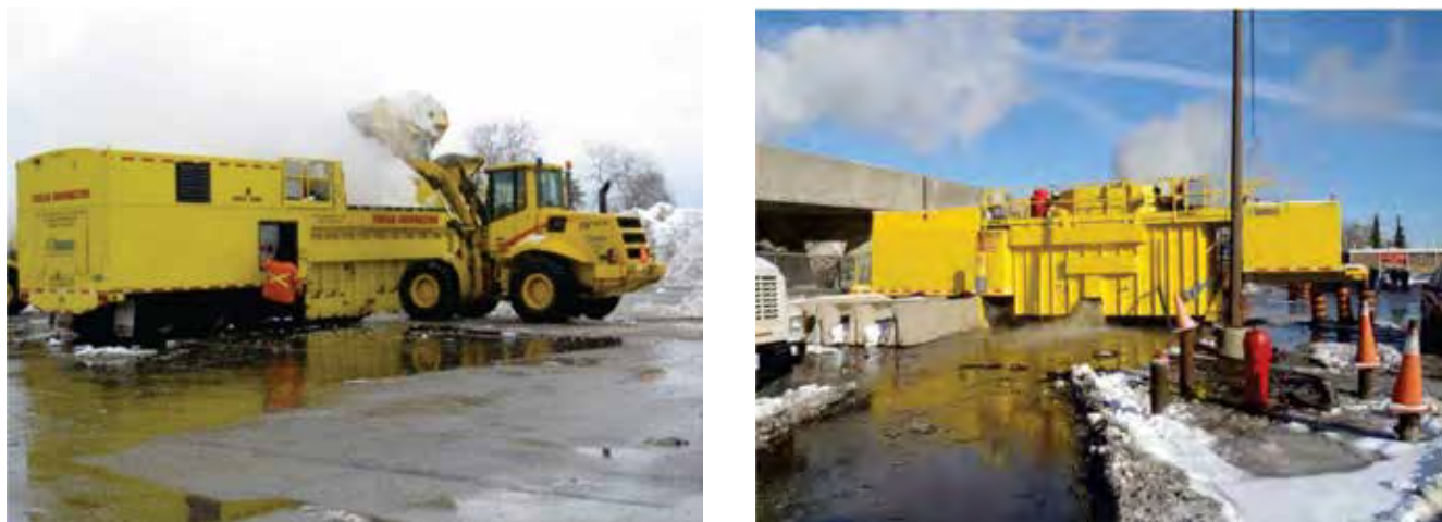
FIGURE B3 (left) A snow melter in use by the city of Toronto staff during the winter of 2007/2008; (right) another snow melter in use by the city of Toronto staff during the winter of 2010/2011 (Photos: City of Toronto, Canada).
