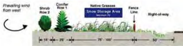
FIGURE 10 Diagram of a living snow fence used by the Iowa DOT Conservation Reserve Program (CRP) (Iowa DOT 2012c).
