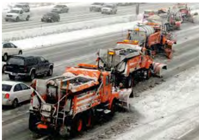
FIGURE 7 Snowplows with hopper-type spreaders (right lanes) and “all-liquid” truck (center lane) (Courtesy: Utah DOT).
