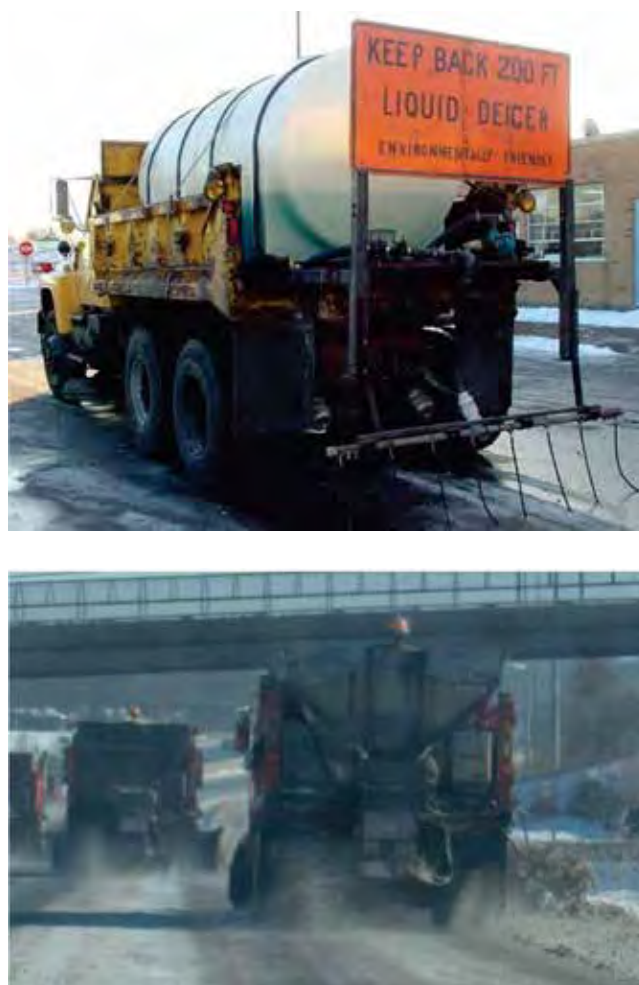
FIGURE 3 Anti-icing (top) and deicing operations (bottom) (Courtesy: Wisconsin and Kansas DOTs, respectively).
