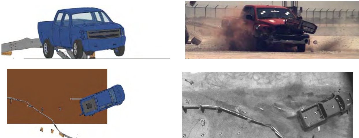
FIGURE 1 Simulations were used to determine the farthest downstream initial impact location that could guarantee the redirection of a 5,000-lb (2,270-kg) pickup truck.
