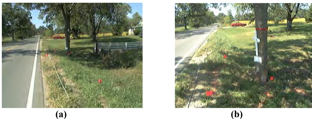
FIGURE 5 1999 Pontiac Grand Am collision with 16-in. diameter tree: (a) tree located 10 ft from travel lane and (b) tree was rigid; no detectable damage. (NASS–CDS 1999-11-133)
