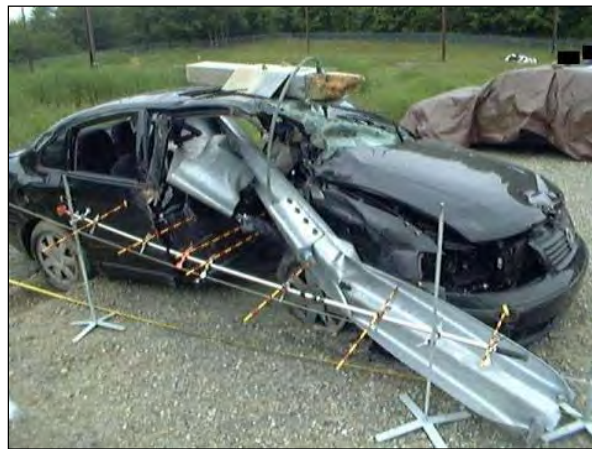
FIGURE 9 Fatal nontracking side impact into a guardrail end terminal.
