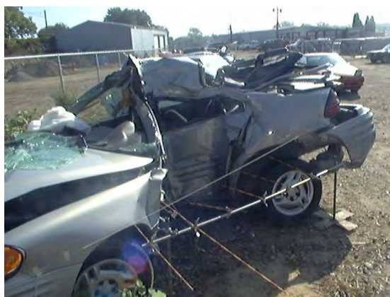
FIGURE 4 1999 Pontiac Grand Am after side crash with tree (NASS–CDS 1999-11-133).
