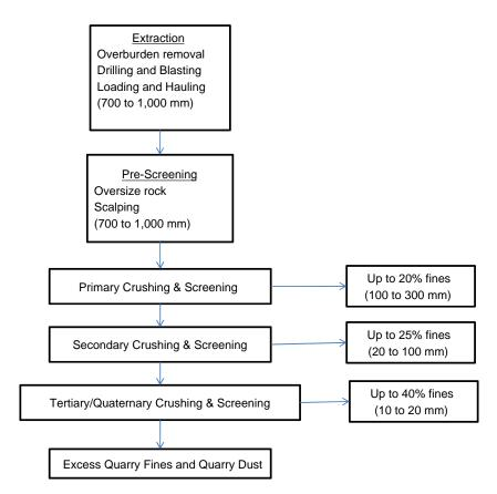
FIGURE 5 Flowchart for a typical quarry operation (RMRC 2008).
