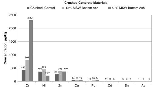
FIGURE 3 Elements leached from crushed concrete (after Aubert et al. 2004).
