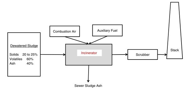
FIGURE 6 Schematic of sewage sludge combustion process (RMRC 2008).
