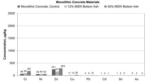
FIGURE 2 Elements leached from monolithic concrete samples (after Aubert et al. 2004).
