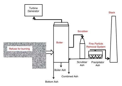
FIGURE 1 Schematic for MSW combustion process.
