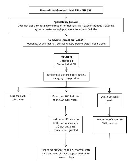
FIGURE 14 NR 538 Unconfined Geotechnical Fill Section 538.8 (after WE Energies 2004).
