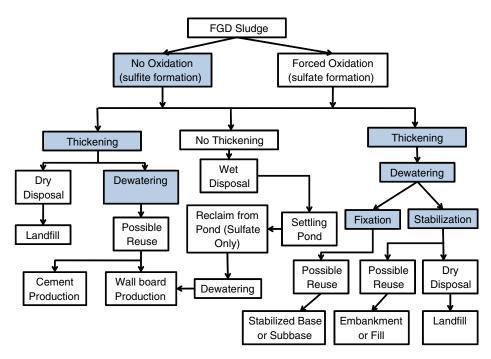
FIGURE 10 Flow chart for FGD sludge to product or landfill (after RMRC 2008).
