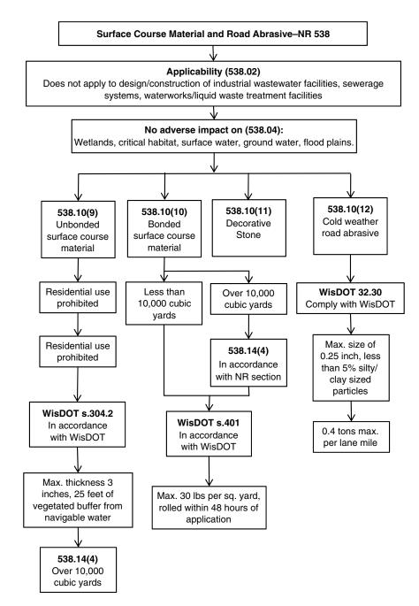
FIGURE 15 NR 538 Surface Course Material and Road Abrasive Sections 538.9 through 538.12 (after WE Energies 2004).
