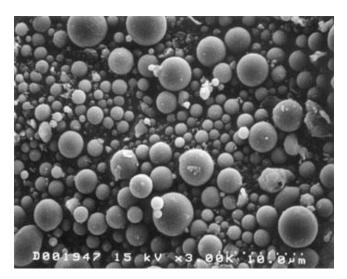
FIGURE 5 Fly ash at 2,000× magnification (FHWA and ACAA 2003).
