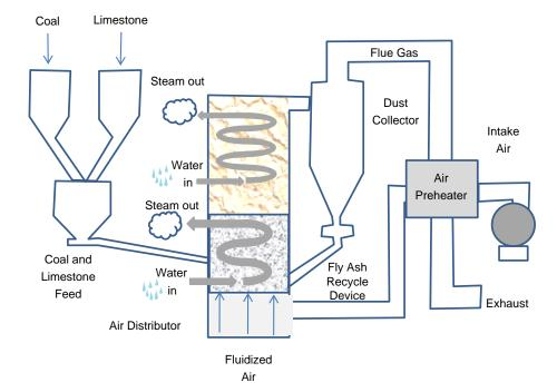
FIGURE 3 Schematic of a fluidized bed combustion boiler (EERC 2009).
