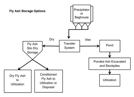
FIGURE 2 Fly ash storage options (continued from previous figure; after FHWA 2005).
