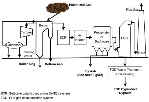
Schematic after Using Coal Ash in Highway Construction: A Guide to Benefits and Impacts. EPA April 2005
