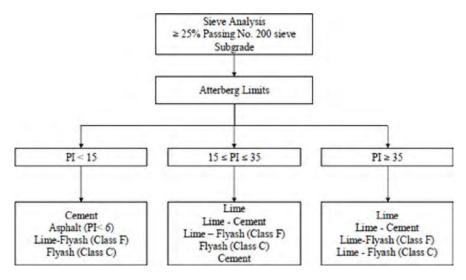
FIGURE 11 Flow chart for selecting additive for stabilizing soils (after Little and Nair 2009).
