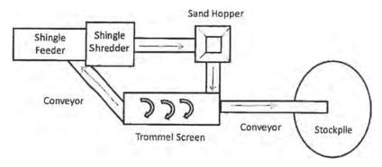
FIGURE 19 Typical grinding operation set up (after Brock 2007).
