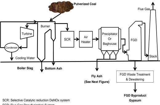
FGD: Flue Gas Desulfurization System
