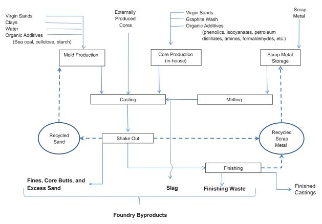
FIGURE 21 Flow chart for the generation of foundry sand byproducts (after Partridge and Alleman 1998).
