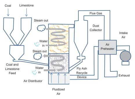
FIGURE 3 Schematic of a fluidized bed combustion (FBC) boiler (EERC 2009).
