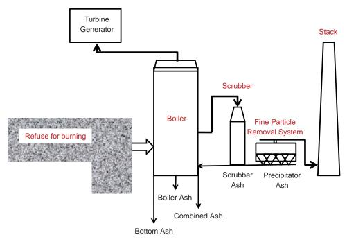
FIGURE 5 Schematic for MSW combustion process (after RMRC 2008).
