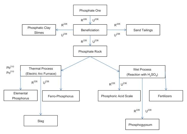
FIGURE 24 Schematic of phosphate process (after Deshpande 2003).
