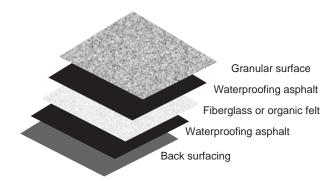
FIGURE 18 Typical composition of roofing shingles (after Gevrenov 2007).
