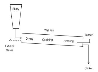
FIGURE 15 Typical long-wet kiln configurations (after "Understanding Cement" 2010).
