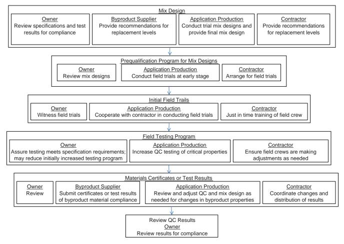
FIGURE 25 Example of QC program sequence when using byproducts in highway applications (after Bouzoubaâ and Fournier 2003, 2005).
