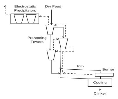
FIGURE 16 Precalciner kiln configuration (after "Understanding Cement" 2010).
