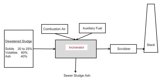
FIGURE 6 Schematic of sewage sludge combustion process (RMRC 2008).
