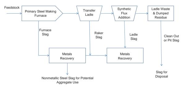
FIGURE 10 Slag production from steel making plant (after RMRC 2008).
