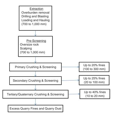
FIGURE 8 Flowchart for a typical quarry operation (RMRC 2008).
