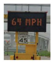
(b) Radar-Activated Portable Changeable Message Sign
