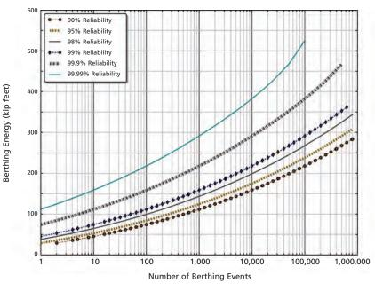
FIGURE 2 Impact energy design chart: reliability plot showing lognormal berthing energy in relation to number of berthing events.
