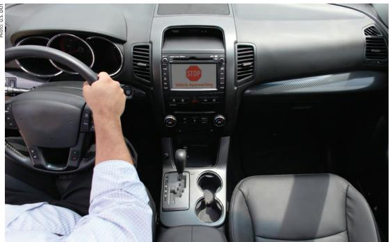
Among the in-vehicle safety devices is a forward collision warning, which alerts the driver to a stopped or slow vehicle ahead.
