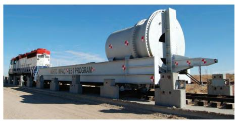
Full-scale tank car impact test setup for evaluating safety improvements under the Next-Generation Railroad Tank Car project at the Transportation Technology Center near Pueblo, Colorado.
