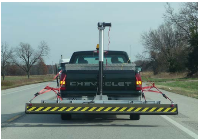
Figure 3.1. 3d-Radar equipment used for field tests.
