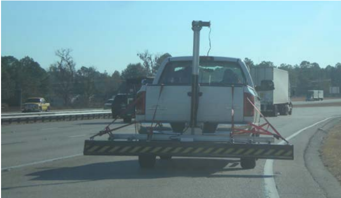
Figure 1.1. 3d-Radar equipment used for field tests.
