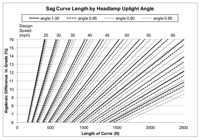
Figure 19. Curve lengths by headlamp uplight angle.
