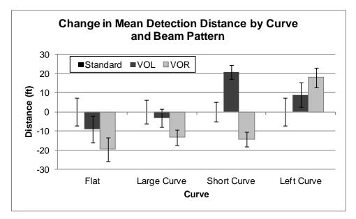
*Figure 36. Change in mean detection distance by curve and beam pattern.*
