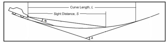
Figure 2. Sight distance and curve length on a sag curve.
