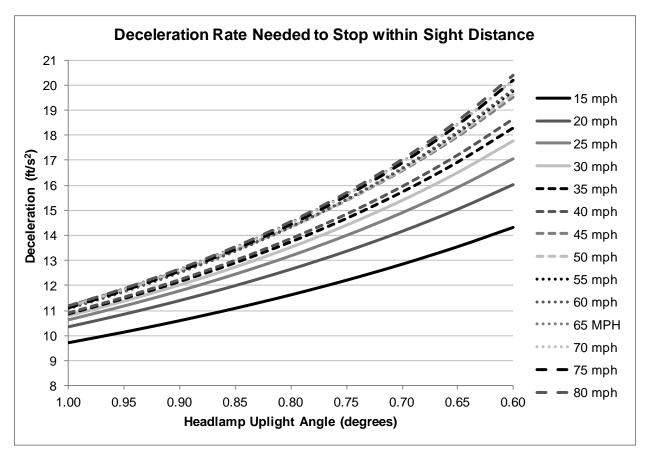
Figure 20. Desired deceleration rate by design speed.
