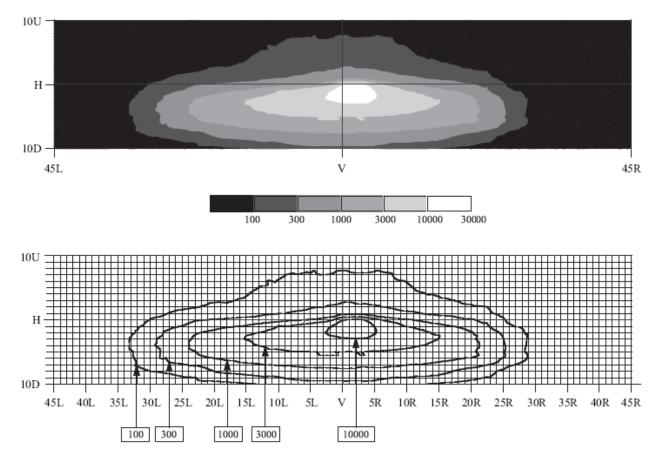
Figure 8. Isocandela diagrams of the median luminous intensities for sales-weighted sample representing the low-beam headlamps on current passenger vehicles in the U.S. The two panels represent the same information in two different formats. Maximum intensity: 22740 cd at 1.0°R, 1.0°D. (Test voltage:12.8V) (Source: Schoettle et al., 2004).
