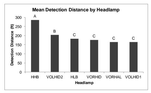
Figure 27. Mean detection distance by headlamp.
