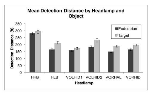
Figure 30. Mean detection distance by headlamp and object.
