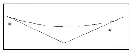
Figure 1. Type III sag vertical curve.
