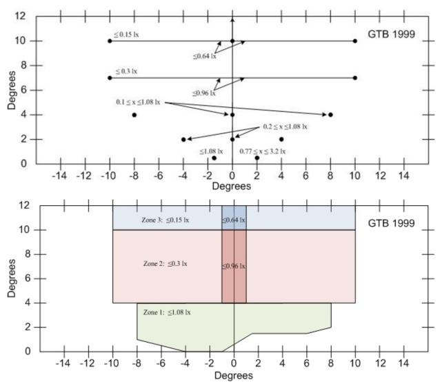
*Figure 7. Test points (top) and zones (bottom) of the harmonized beam pattern proposed by the GTB.*
