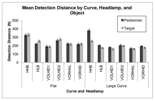
*Figure 32. Mean detection distance by curve, headlamp, and object.*
