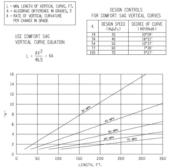
*Figure 13. Design controls for comfort sag vertical curves. (Source: Road Design Manual, Chapter 3-4, Vertical Alignment, Minnesota Department of Transportation, 2004, Page 3-4(12)).*
