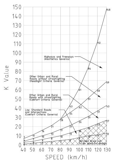
Figure 18. Minimum K values for sag curves (Source: Austroads, 2010, Figure 8.7).
