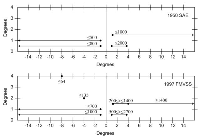
Figure 4. Light allowed above horizontal by SAE standards.
