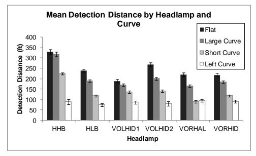
Figure 31. Mean detection distance by headlamp and curve.
