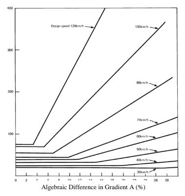
Figure 17. Length of sag vertical curves L (m) for adequate comfort (Source: Overseas Road Note 6, 1998).
