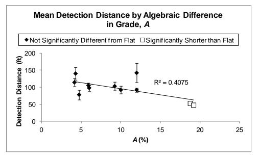
Figure 41. Mean detection distance by algebraic change in grade.
