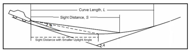
Figure 3. Sight distance and curve length on a sag curve.
