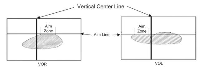
Figure 6. Beam patterns and aiming positions for VOR and VOL headlamps (Source: Headlamp Aiming Procedure, 2006).
