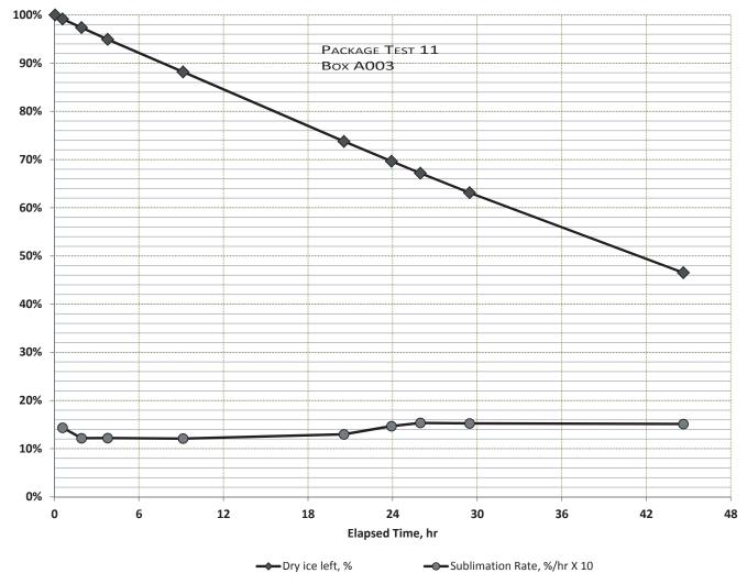
Figure 6. Representative package test results.
