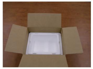
Battelle photo Figure 3. Inside view of insulated shipping carton.
