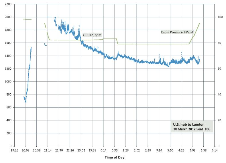
Figure 13. Cabin carbon dioxide concentration on outbound flight.
