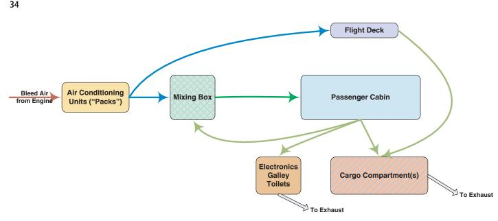
Figure 9. General ventilation air flows in an aircraft.
