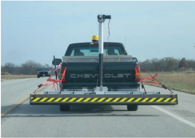
Figure A.1. Example of full lane width GPR antenna array.
