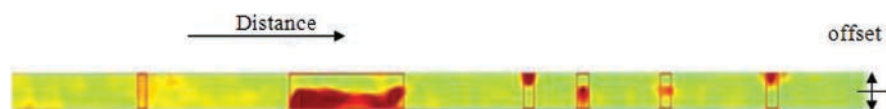
Figure 3.22. Red rectangles showing final output of algorithm, identifying locations with potential delamination.
