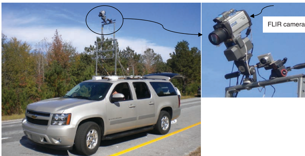
Figure 3.11. Infrared thermography setup for testing at the NCAT Pavement Test Track.
