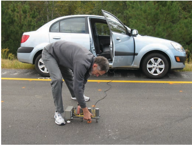
Figure 3.13. PSPA Testing at NCAT Test Track.
