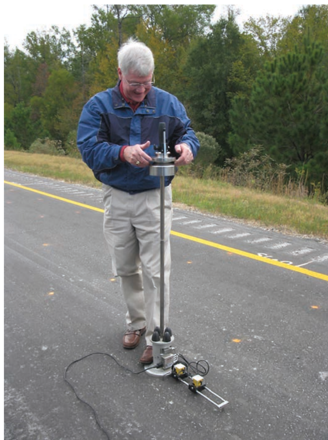
Figure 3.18. LWD testing at NCAT test track.
