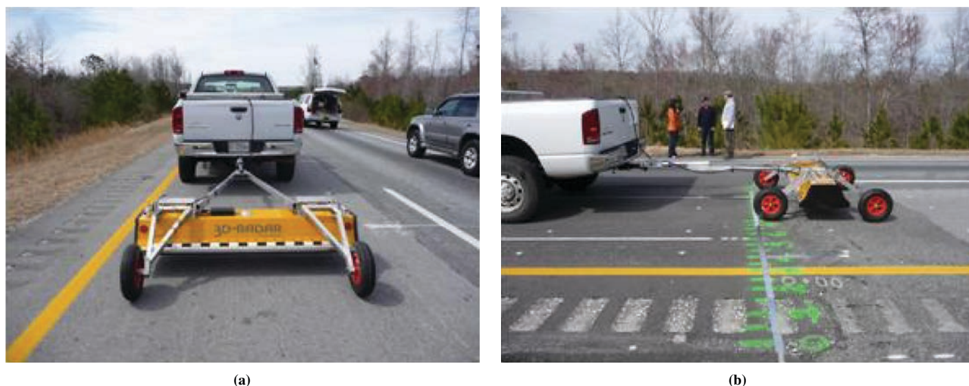
Figure 3.6. 3d-Radar swept frequency (150 MHz to 3 GHz) noncontact array: (a) rear view and (b) side view.
