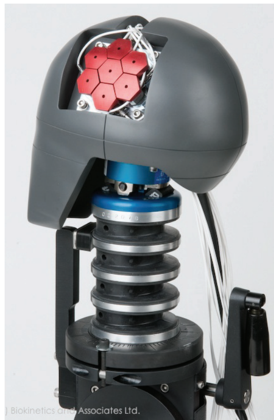
FIGURE 10-3 (a) The University of Virginia's Hybrid III head model used for laboratory simulations and measurements. (b) Biokinetics headform variant of the Hybrid III headform for ballistic impact. SOURCE: Courtesy of Biokinetics and Associates, Ltd.
