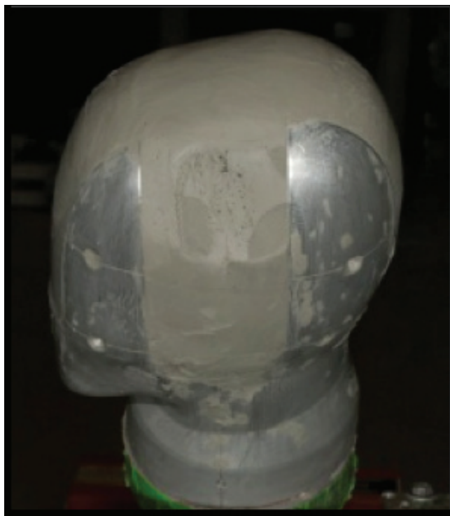
FIGURE D-9 Example of headform showing a penetration as evidenced by the presence of projectile fragments in the clay. SOURCE: ATC (2013).
