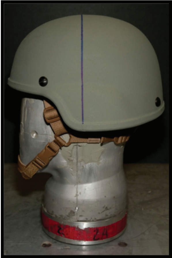
FIGURE D-7 Helmet mounted on a headform. SOURCE: ATC (2013).
