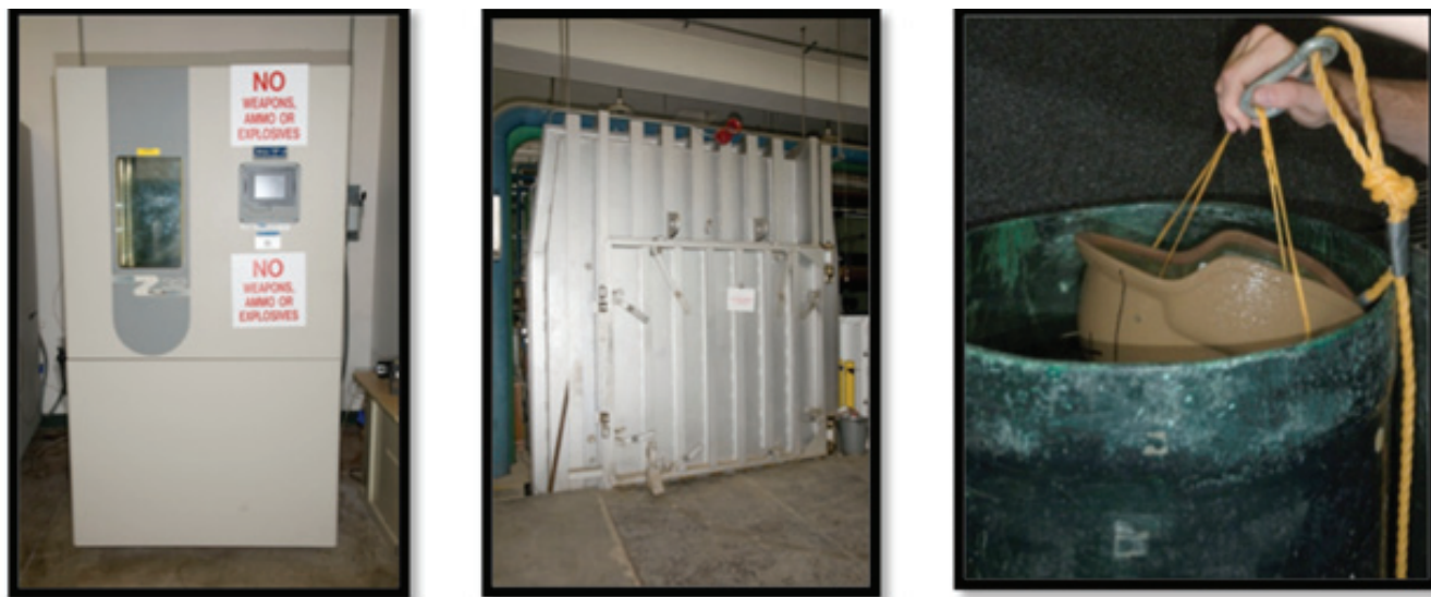
FIGURE D-16 Examples of helmet conditioning. SOURCE: Kyle Markwardt, Test Officer, Aberdeen Test Center, “Helmet IOP PED-003 Briefing to NRC Helmet Protocols Committee,” presentation to the committee on March 22, 2013.
