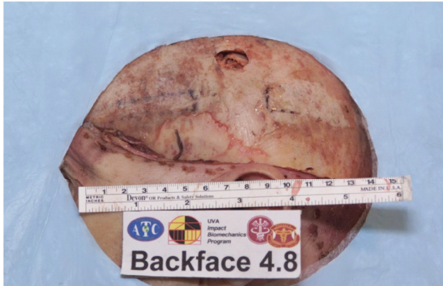
FIGURE 3-4 Long linear and depressed skull fractures from non-penetrating helmet BFD in a human cadaveric model. SOURCE: Bass et al. (2003).
