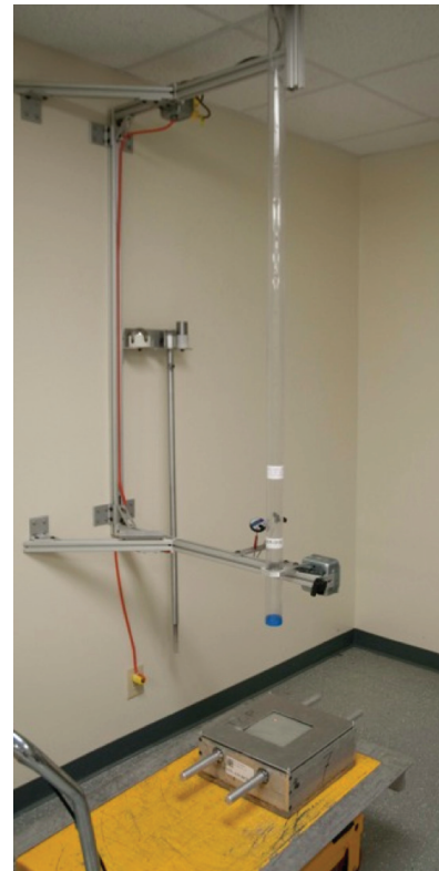
FIGURE D-15 Clay calibration test rig. SOURCE: ATC (2013).
