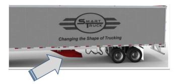
FIGURE 6-8 SmartTruck undertray: UT-1. Available at http:// smarttrucksystems.com/undertray-UT1Base.php. Accessed November 14, 2013.
