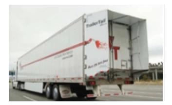
FIGURE 6-9 ATDynamics trailer tail. Available at http://www. atdynamics.com/trailertail.htm. Accessed November 14, 2013.
