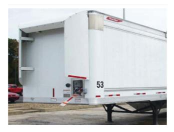
FIGURE 6-6 Trailer front gap fairing. SOURCE: Freight Wing. Available at http://www.freightwing.com/gap\_fairing.php. Accessed November 14, 2013.
