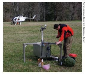
The U.S. Geological Survey worked with the Washington Department of Natural Resources, Washington State DOT, and Snohomish County to assess slope conditions using a remote sensing spider unit.
