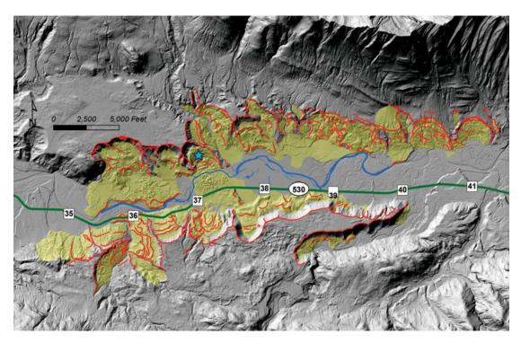
FIGURE 3 Geomorphic map of unstable landforms on a bareearth model derived from airborne lidar collected in 2010 and immediately after the 2014 landslide. Red lines are primary landslide scarps, and yellow shadings are landslide deposits; star denotes initiation zone of the SR-530 landslide (2).
