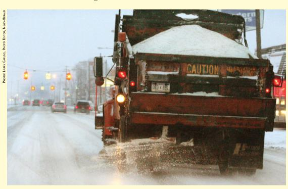
A salt truck applies deicing material before a storm in Wayne County, Michigan. Strict stormwater regulations have caused state DOTs to examine deicing applications that use sodium chloride.
