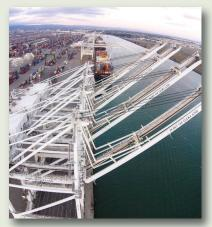
COVER: In 2016, a major expansion of the Panama Canal will facilitate passage of vessels up to 15,000 TEUs and with drafts of 50 feet. The large vessels will require super-post-Panamax crane and draft equipment, shown here at the Port of Oakland. (Photo: Eddie Codel, Port of Oakland)
