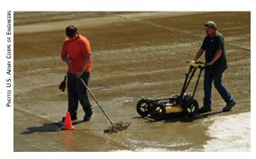
Contractors use a ground-penetrating radar device on the Gavins Point Dam spillway in South Dakota.
