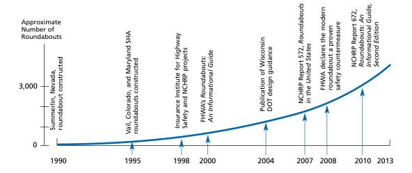
FIGURE 1 Timeline of roundabouts implementation in the United States.
