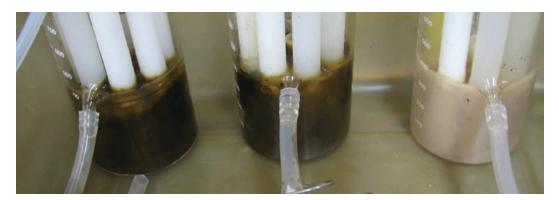
*Figure 5-5. Reactors at the conclusion of the experiment on Day 28. (From left to right, 25 percent full sunlight, 12 percent full sunlight, dark.)*
