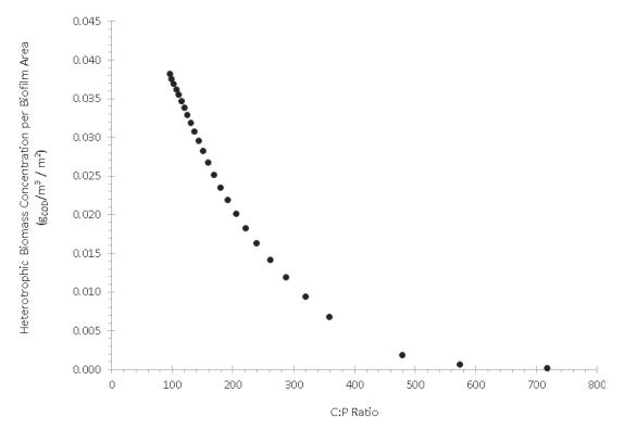
*Figure 5-20.* Heterotrophic organism concentration per unit area in the modeled biofilm as a function of C:P ratio.
