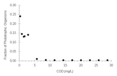
*Figure 5-10. Model projected active fraction of phototrophic organisms over range of COD concentrations with sunlight.*
