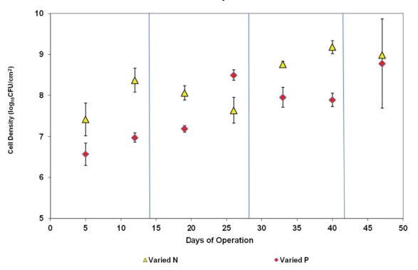
Figure 5-16. Heterotrophic plate counts from biofilm accumulated on coupons in reactors. (Error bars represent  $\pm 1$  standard deviation from the mean. Vertical lines denote times when the varied nutrient concentration was increased [see Table 4-5]).
