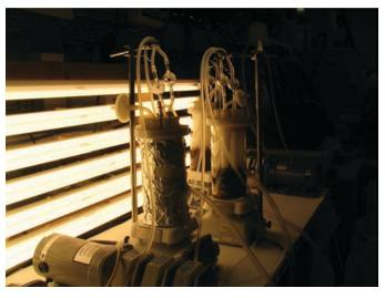
Figure 4-4. Biofilm growth reactors in dark, at 12 percent full sunlight, and at 25 percent full sunlight.
