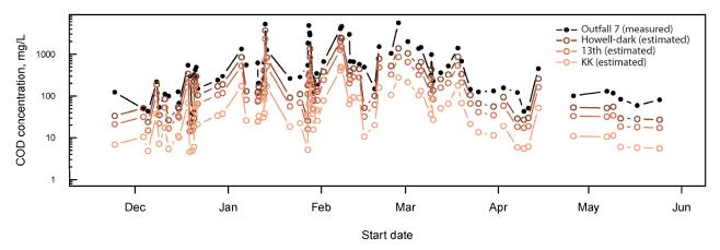
Figure 5-26. Flow-composite COD concentrations from Outfall 7, with estimated flow-composite COD concentrations at downstream monitoring locations. ([a] Flow-composite COD concentrations at Outfall 7 and estimated flow-composite COD concentrations based on measured concentrations in point samples at [b] Howell-dark, [c] 13th, and [d] KK.)
