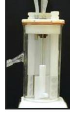
Figure 4-3. CDC biofilm reactor.
