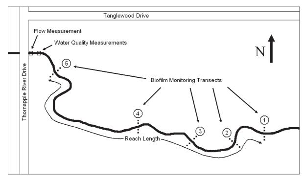
Figure 4-2. Elements of a biofilm monitoring reach.
