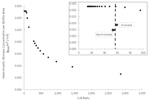
*Figure 5-21.* Heterotrophic organism concentration per unit area in the modeled biofilm as a function of C:N ratio. (Inset shows the lowest portion of the range.)
