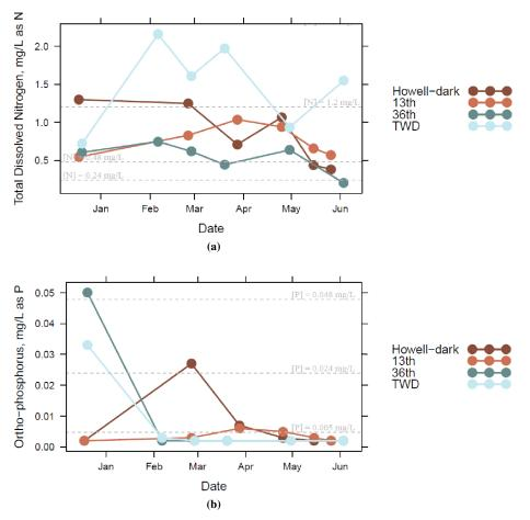
Figure 5-19. Measured total dissolved nitrogen (a) and ortho-phosphorus as P (b) concentrations at water-quality monitoring locations (with lines showing concentrations and ratios used in laboratory tests).
