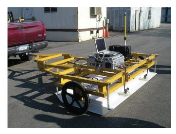
Figure 2.1. UIT's Multichannel GPR system, the TerraVision II.
