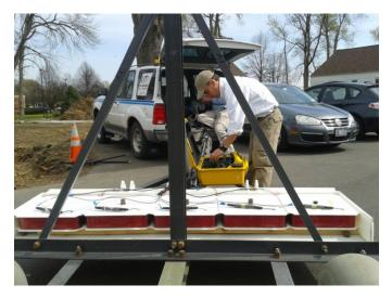
Figure 3.73. Configuration and testing of the 5-by-1 TDEMI sensor array on UIT's metal-free trailer.
