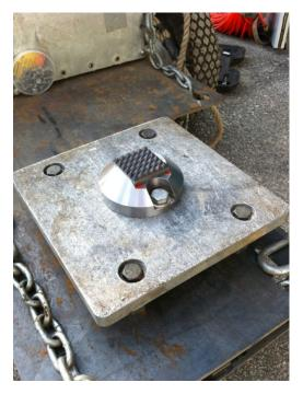
Figure 3.13. Ground coupler base late for MicroVib.
