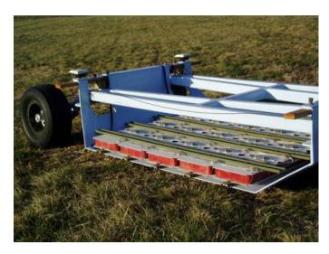
Figure 2.5. SAIC/NRL TDEMI array for buried-object location and classification.
