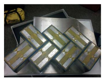
Figure 2.2. Internal arrangement of a single bank of TerraVision II GPR antennas.
