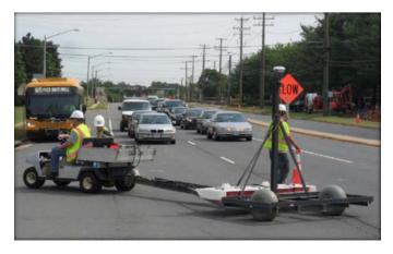
*Figure 3.95. TDEMI prototype data acquisition during in-service testing.*
