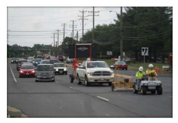
*Figure 3.94. TerraVision II data acquisition during in-service testing.*
