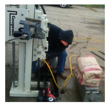
Figure 3.15. Placement of downhole and reference probes during field testing.
