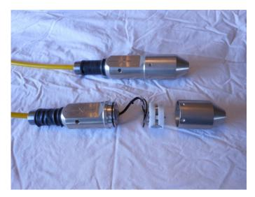
Figure 3.14. Housing probe and triaxial accelerometers.
