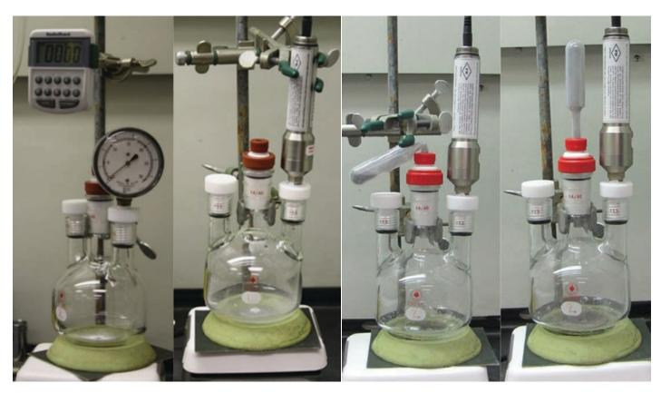
Figure A-4. Complete reaction apparatus with analog gauge and timer for manual data acquisition (far left), with pressure transducer (center left) as configured for use with liquids, with solids addition tube in place (center right) for use with solids, and with solids addition tube after addition of solids (far right).
