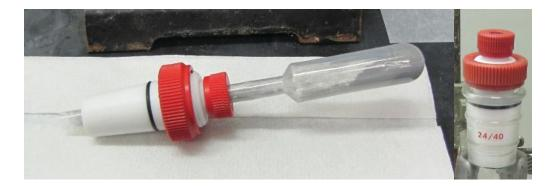
FIG. 3. Detail (left) of a solid addition apparatus and (right) a friction fit closure that accommodates both a septum and provides (via the friction-fit) pressure relief for the test apparatus.
