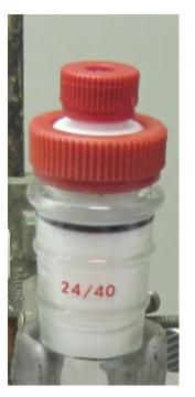
Figure A-6. Detail of liquid addition/septum closure fitting with septum installed (not visible). Note that this is a friction fit closure of the vessel.
