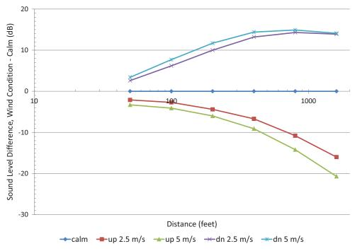
Figure 52. Sound-level difference without noise barrier and varying wind and calm conditions (automobiles and trucks, 5-ft receiver, and soft ground).
