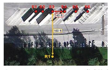
Figure 25. Geometry for comparing array of individual noise sources to a single line source.<sup>13</sup>
