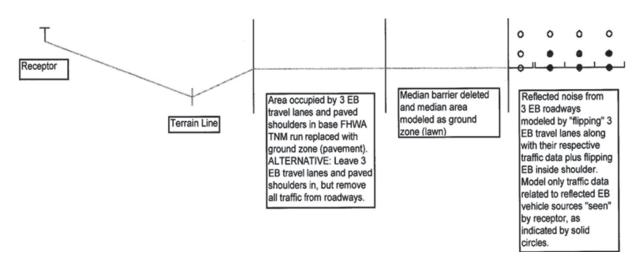
Figure 32. Skew section of reflected (flipped) FHWA TNM run.
