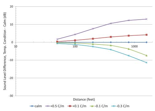
*Figure 54. Sound-level difference without noise barrier, varying temperature, and calm conditions (automobiles and trucks, 5-ft receiver, and soft ground).*
