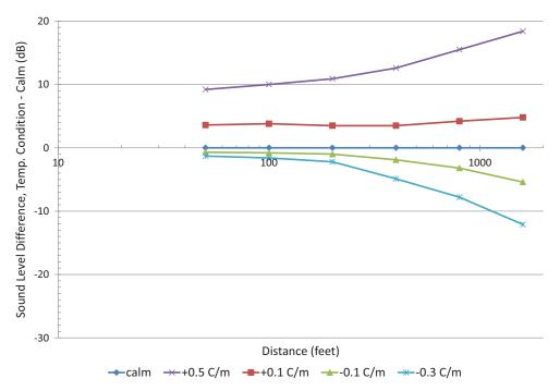
*Figure 53. Sound-level difference with noise barrier, varying temperature, and calm conditions (automobiles and trucks, 5-ft receiver, and soft ground).*
