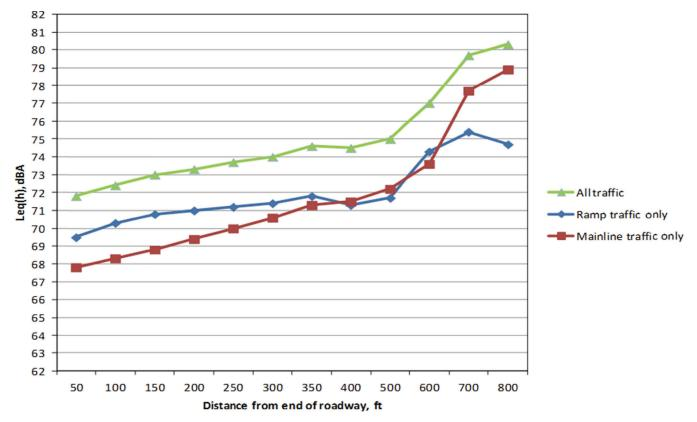
Figure 11. Diamond interchange  $L_{eq}(h)$  for ramp traffic equal to 25% of mainline traffic using NCHRP Report 311 deceleration roadway segment lengths and speeds, for a series of receivers offset 50 ft from the ramp centerline.
