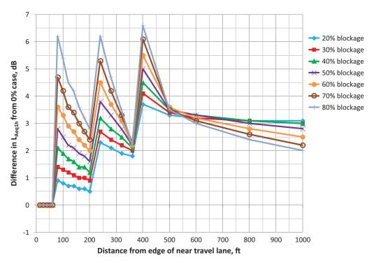
*Figure 39.* Noise reduction as a function of building percentage for three 20-ft-high building rows near a single 12-ft-wide roadway.
