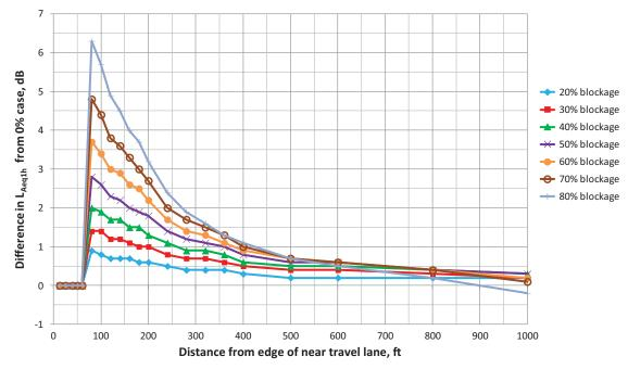
*Figure 34.* Noise reduction as a function of building percentage for a single 20-ft-high building row 70 ft from edge of an eight-lane roadway.
