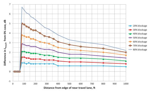
*Figure 35.* Noise reduction as a function of building percentage for a single 30-ft-high building row 70 ft from edge of an eight-lane roadway.
