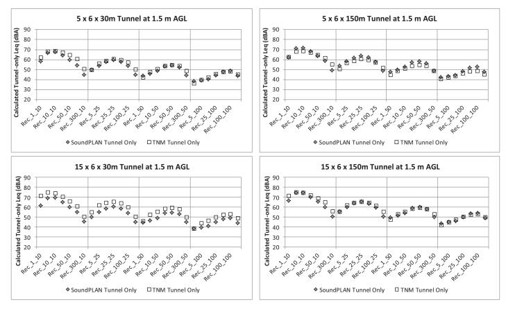
Figure 66. TNM and SoundPLAN tunnel-only noise levels for three parallel roads inside the tunnel, each with 2.5 × the volume of road outside tunnel—at distances of 1, 5, 10, 25, 50, 100, and 300 m from the tunnel opening and 10, 25, 50, and 100 m from the road centerline and 1.5 m AGL.
