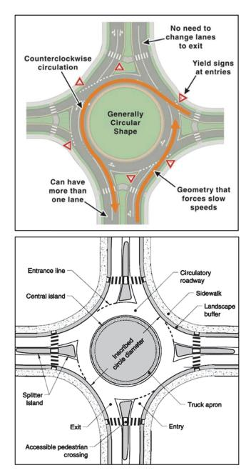
Figure 5. Modern roundabout characteristics.8
