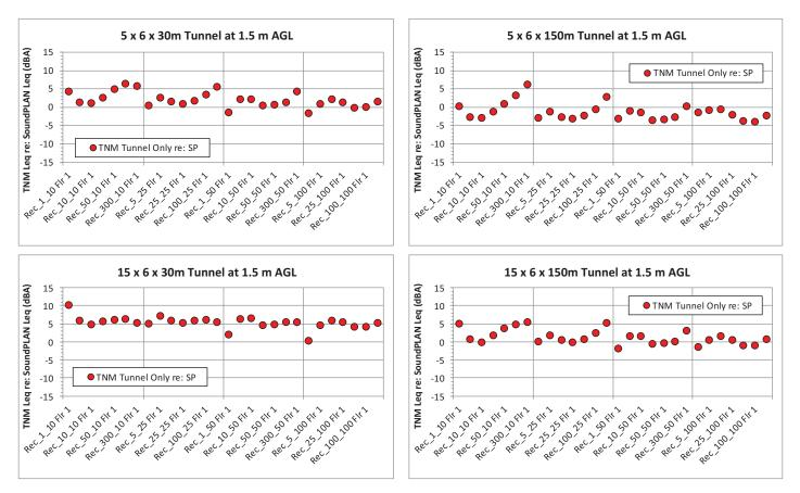
Figure 67. TNM tunnel-only noise level minus SoundPLAN tunnel-only noise level for three parallel roads inside the tunnel, each with 2.5 × the volume of road outside tunnel—at distances of 1, 5, 10, 25, 50, 100, and 300 m from the tunnel opening and 10, 25, 50, and 100 m from the road centerline and 1.5 m AGL.
