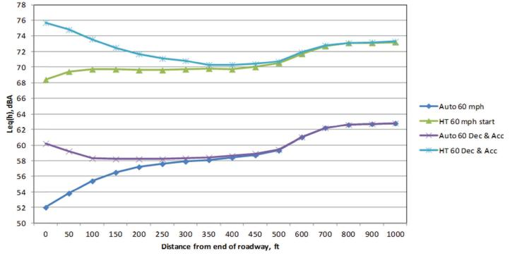
Figure 9. Separate  $L_{eq}(h)$  for 1,000 automobiles and 1,000 heavy trucks decelerating from 60 mph to 0 mph using NCHRP Report 311 roadway segment lengths and speeds and then accelerating downstream from 0 mph to 60 mph for a series of receivers offset 100 ft from the deceleration roadway.
