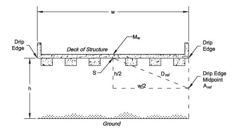
h = Height of structure, from ground to underside of deck
