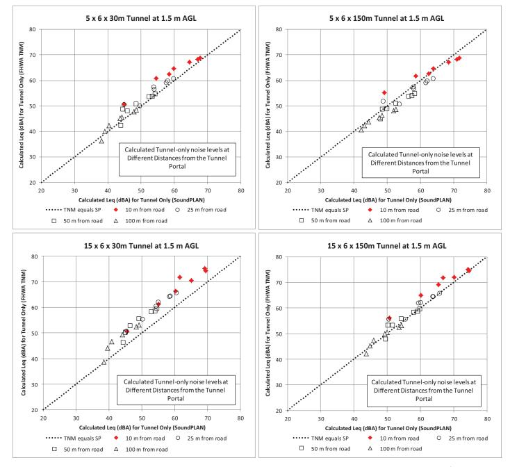
Figure 68. FHWA TNM tunnel-only noise levels plotted against SoundPLAN tunnel-only noise levels for three parallel roads inside the tunnel, each with 2.5 × the volume of road outside tunnel—at distances of 1, 5, 10, 25, 50, 100, and 300 m from the tunnel opening and 10, 25, 50, and 100 m from the road centerline and 1.5 m AGL.
