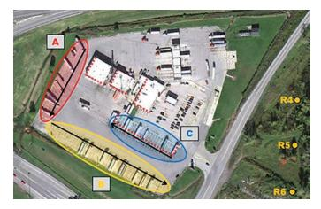
Figure 30. Example 6—truck stop with buildings and truck trailers as noise barriers.<sup>21</sup>
