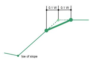
Figure 47. Section view of flat-top berm shape including the suggested "rounding off" of the top edge.
