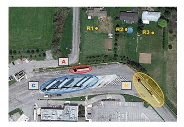
Figure 27. Example 2—multiple idling trucks at service plaza modeled as line sources.<sup>17</sup>
