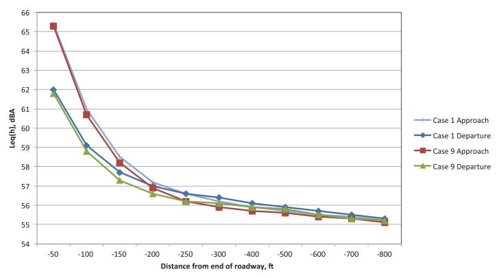
Figure 23. Comparison of  $L_{eq}(h)$  for Cases 1 and 9 for a series of receivers offset 200 ft from the western leg roadways for 1,000 automobiles approaching and departing roundabout at 40 mph.
