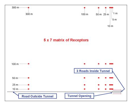
Figure 62. Plan view of modeled geometry for tunnel measuring 15 by 6 by 30 m with three parallel and evenly spaced roads inside (with the 5-by-7 matrix of receptors).
