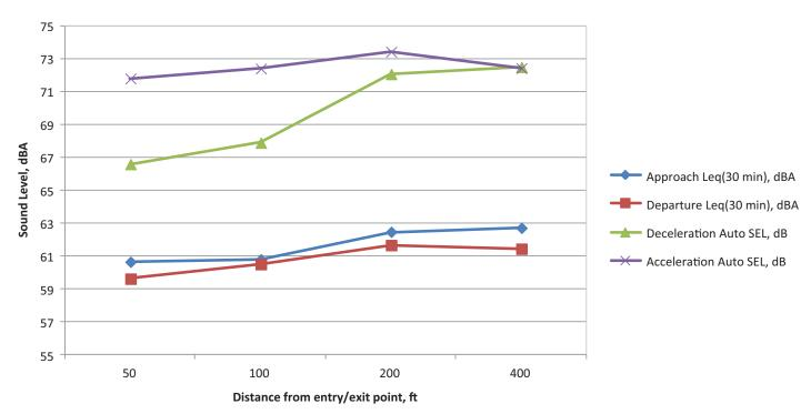
Figure 24. Measured L<sub>eq</sub> (30 min) at 25-ft offset from edge of travel lane, Liberty Pike roundabout.
