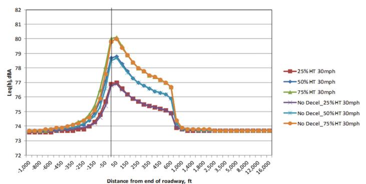
Figure 18.  $L_{eq}(h)$  for 1,000 heavy trucks for one-way "Deceleration + Cruise" compared to "All Cruise" on the upstream deceleration side for a 30-mph cruise speed and an array of receivers at a 50-ft offset distance from the roadway.
