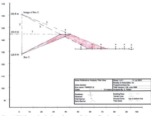
Figure 1. TNM skew section showing roadways contributing to reflected sound.<sup>2</sup>
