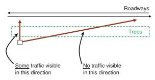
Figure 48. Roadway visibility through a narrow tree belt.
