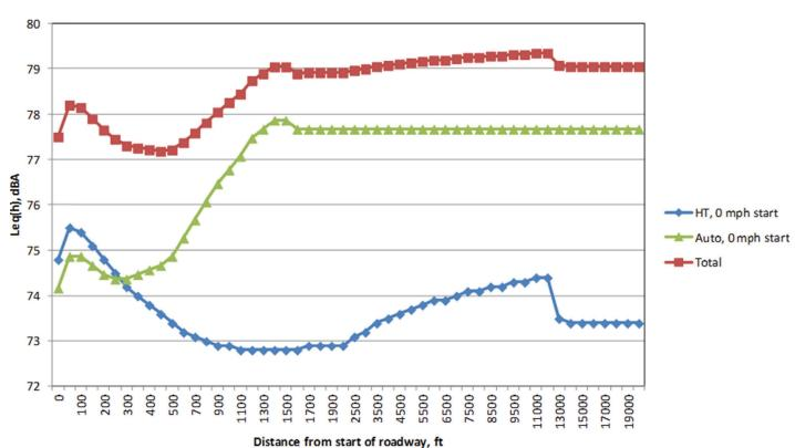
Figure 8.  $L_{eq}(h)$  for 97% automobiles and 3% heavy trucks (31,000 vehicles), accelerating from 0 mph to 60 mph with 100% of the Vehicles Affected and a Speed Constraint of 0 mph for a series of receivers offset 100 ft from the roadway.
