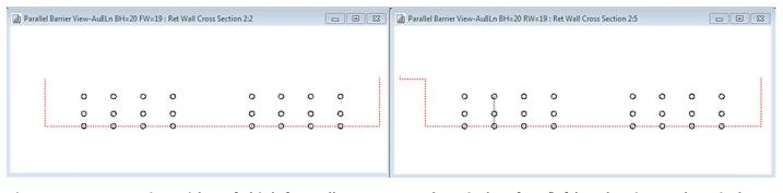
Figure 61. Cross section with 19-ft-high far wall as an external vertical surface (left) and an internal vertical surface with a 1-ft noise barrier offset 10 ft from the top of the internal vertical surface (right).
