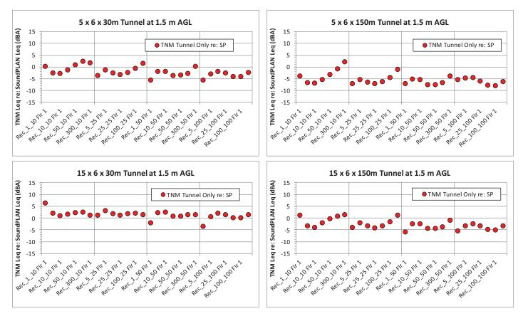
Figure 64. TNM tunnel-only noise level minus SoundPLAN tunnel-only noise level for three parallel roads inside the tunnel, each with  $1 \times$  the volume of road outside tunnel—at distances of 1, 5, 10, 25, 50, 100, and 300 m from the tunnel opening and 10, 25, 50, and 100 m from the road centerline and 1.5 m AGL.
