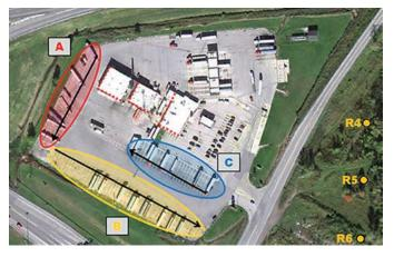
Figure 29. Example 5—truck stop with buildings as fixed-height noise barriers.<sup>19</sup>
