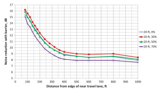
*Figure 41.* Noise reduction for a 20-ft-high noise barrier along the edge of the shoulder of an eight-lane roadway with a 30-ft-high building row located 70 ft from the edge of the near travel lane, for various building percentages.
