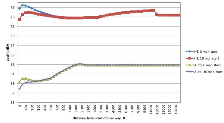
Figure 7.  $L_{eq}(h)$  for 1,000 automobiles and 1,000 heavy trucks, plotted separately, accelerating from 0 mph to 60 mph with 100% of the Vehicles Affected and Speed Constraint of 0 and 10 mph for a series of receivers offset 100 ft from the roadway.
