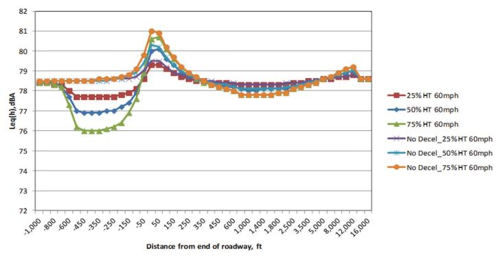
Figure 19.  $L_{eq}(h)$  for 1,000 heavy trucks for one-way "Deceleration + Cruise" compared to "All Cruise" on the upstream deceleration side for a 60-mph cruise speed and an array of receivers at a 50-ft offset distance from the roadway.
