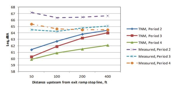
Figure 10. Comparison of measured traffic noise and modeled noise excluding mainline heavy trucks, Briley Parkway exit ramp site.
