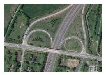
Figure 13. Folded diamond interchange.<sup>12</sup>
