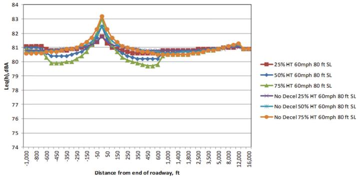
Figure 20.  $L_{eq}(h)$  for 1,000 heavy trucks for two-way "Deceleration + Cruise" compared to "All Cruise" on the upstream deceleration side for a 60-mph cruise speed and an array of receivers at a 50-ft offset distance from the roadway.
