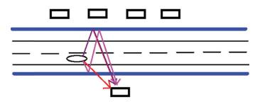
*Figure 56. Plan view of multiple reflections off parallel highway noise barriers.*
