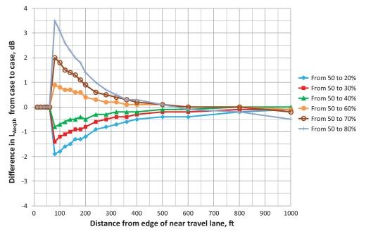
*Figure 36. Differences in noise reduction for various building percentages compared to 50% blockage for a single 20-ft-high building row 70 ft from the edge of an eight-lane roadway.*
