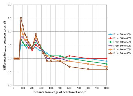
Figure 38. Differences in noise reduction for 10% incremental increases of building percentage for two 20-ft-high building rows near a single 12-ft-wide roadway.
