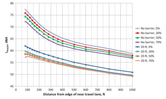
Figure 40. Sound level with and without a 20-ft-high noise barrier along the edge of the shoulder of an eight-lane roadway with a 30-ft-high building row located 70 ft from the edge of the near travel lane, for various building percentages.
