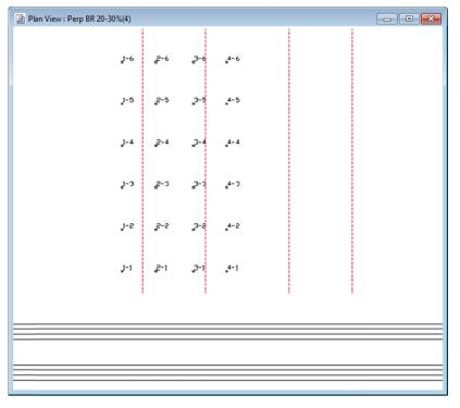
*Figure 42. FHWA TNM plan view of four perpendicular building rows adjacent to an eight-lane highway.*
