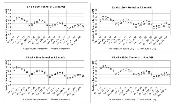
Figure 63. TNM and SoundPLAN tunnel-only noise levels for three parallel roads inside the tunnel, each with  $1 \times$  the volume of road outside tunnel—at distances of 1, 5, 10, 25, 50, 100, and 300 m from the tunnel opening and 10, 25, 50, and 100 m from the road centerline and 1.5 m AGL.
