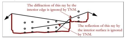
Figure 60. Text and diagram from TNM FAQs on parallel barriers.<sup>59</sup>
