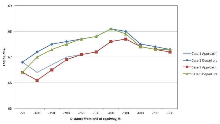
Figure 22. Comparison of  $L_{eq}(h)$  for Cases 1 and 9 for a series of receivers offset 50 ft from the western leg roadways for 1,000 automobiles approaching and departing roundabout at 40 mph.
