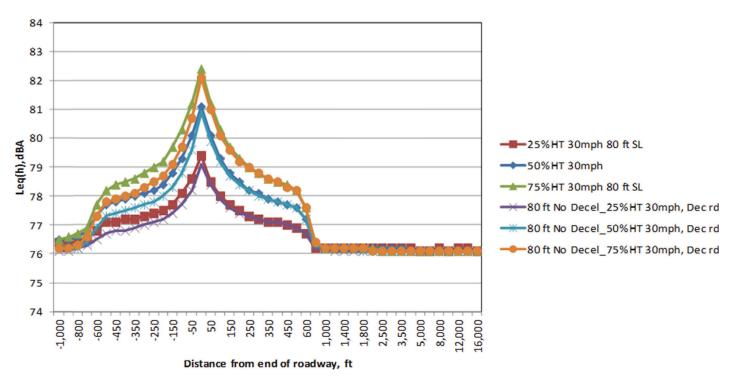
Figure 17.  $L_{eq}(h)$  for 1,000 heavy trucks for two-way "Deceleration + Cruise" compared to "All Cruise" on the upstream deceleration side for a 30-mph cruise speed and an array of receivers at a 50-ft offset distance from the roadway.
