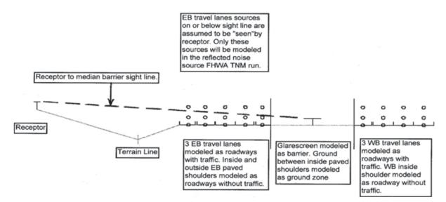
Figure 31. Skew section of base FHWA TNM run.
