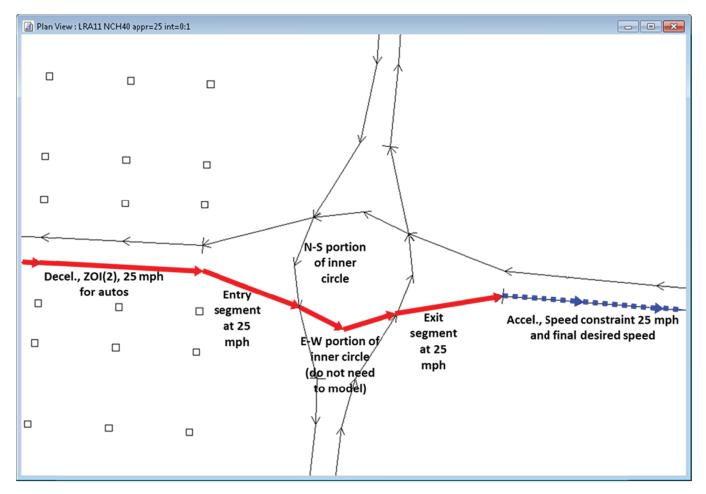
Figure 21. Modeling methodology for eastbound approach and departure legs and center circle of roundabout.
