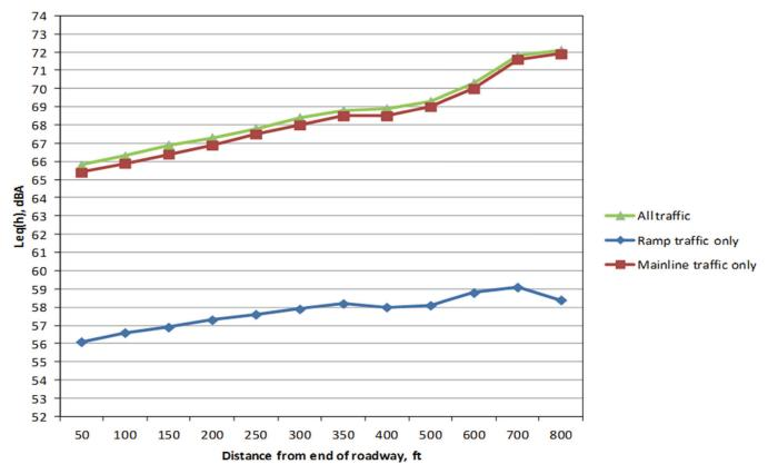
Figure 12. Diamond interchange  $L_{eq}(h)$  for ramp traffic equal to 12.5% of mainline traffic using NCHRP Report 311 deceleration roadway segment lengths and speeds, for a series of receivers offset 200 ft from the ramp centerline.
