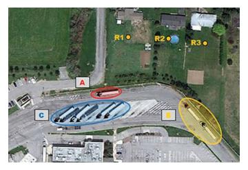
Figure 26. Example 1—idling trucks at service plaza modeled individually.<sup>16</sup>
