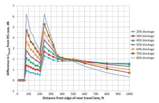
*Figure 37.* Noise reduction as a function of building percentage for two 20-ft-high building rows near a single 12-ft-wide roadway.
