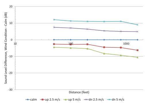
*Figure 51. Sound-level difference with noise barrier and varying wind and calm conditions (automobiles and trucks, 5-ft receiver, and soft ground).*
