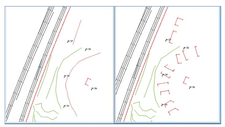
Figure 44. TNM plan view with building rows (left) and building barriers (right), Noise Study Area G of US 29 widening.
