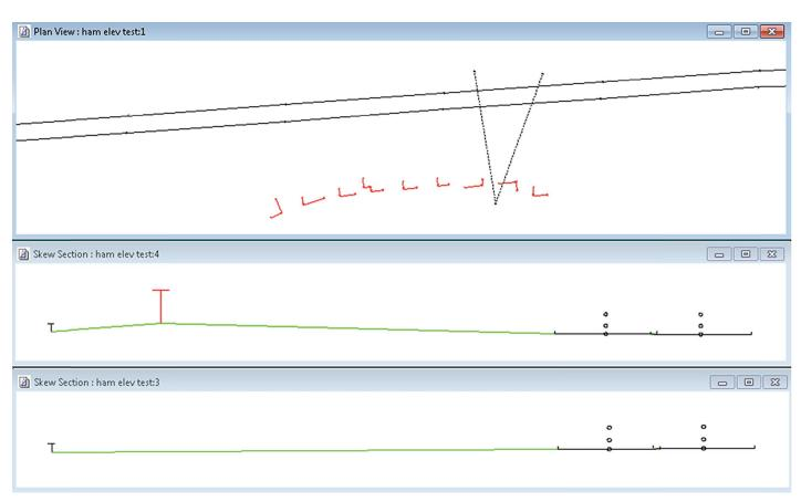
Figure 46. FHWA TNM plan view (top) and skew section views through a building barrier (middle) and through a gap (bottom) where the ground elevation has not been defined.
