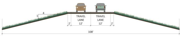
physical size of the roadway prism footprint and the additional impervious area the alternative would add to account for the potentially negative impact of additional stormwater runoff into the adjacent wetlands.
