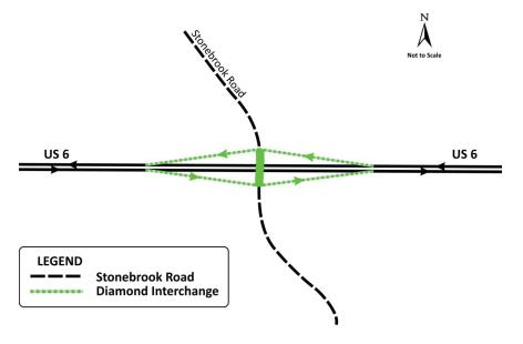
*Interchange Form Alternatives.* This subsection presents schematics of the three alternative interchange forms:
