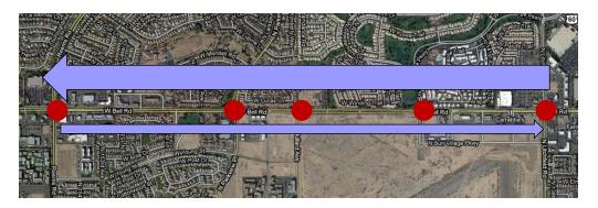
Figure 159. Illustration of relative flows along the arterial during P.M. peak
