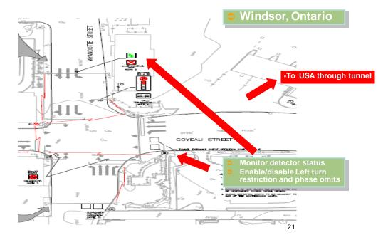
Figure 143. Detail of detector deployment and operational strategies at Tunnel entrance
