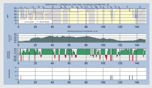
Figure 2-2-5. Speed profile, elevation, train controls (selected freight train).
