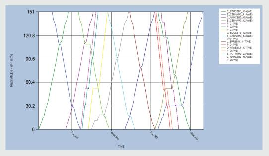
Figure 2-2-2. String chart (alternate case—including passenger trains).
