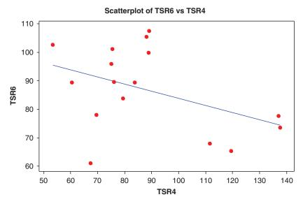
FIGURE 6 Comparison of 4-in. Marshall versus 6-in. gyratory TSR results. (*Source*: Watson et al. 2008b.)
