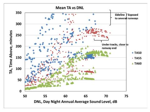
Figure 9 Time Above Different Threshold Levels versus DNL
