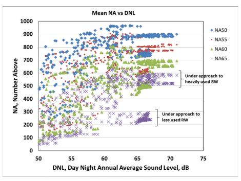
Figure 8 Number Above Different Threshold Levels versus DNL
