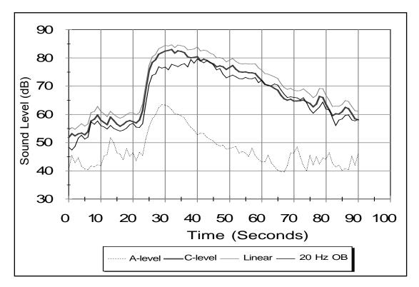
Figure 7 Time Histories of a Single Jet Takeoff as Recorded ~ 3200 Feet Adjacent the Runway
