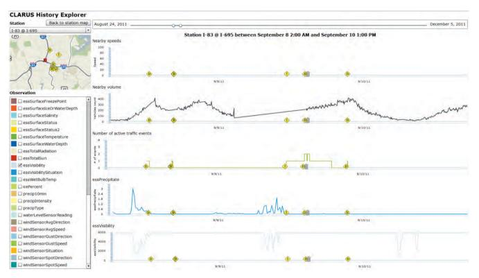
FIGURE A14 An RWIS data explorer allows an agency to see how localized weather, visibility, surface temps, etc., can affect traffic speeds, volumes, and accidents near RWIS stations.
