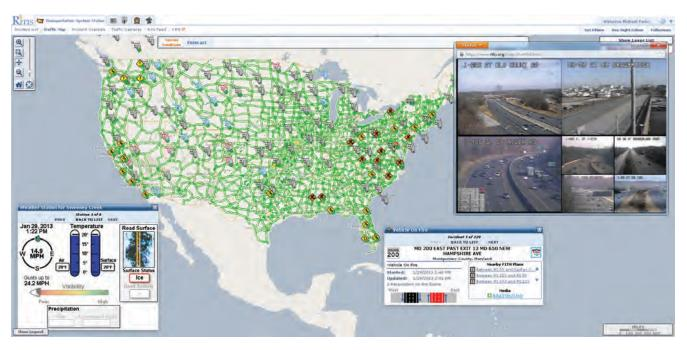
FIGURE A3 A high level screenshot of the real-time RITIS user interface showing several layers of data visualization from comparative traffic flow, to weather, incidents, and even CCTV.
