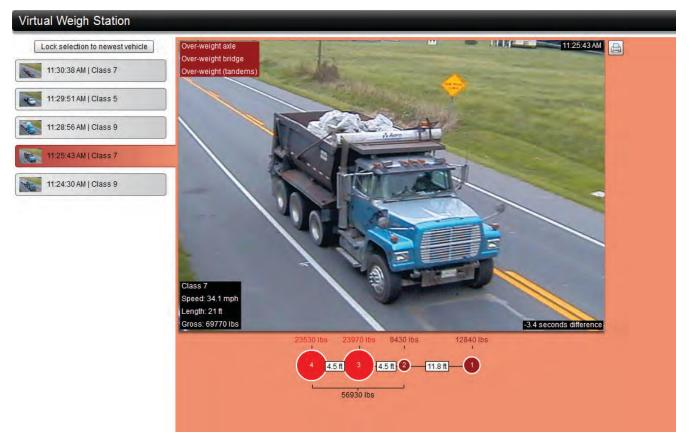
FIGURE A7 Virtual weigh station sensors are visualized within RITIS—axle spacing, axle weights, and other measurements help to target enforcement activities.
