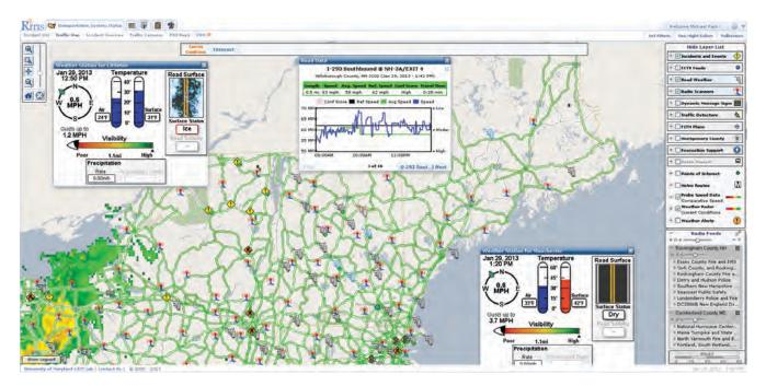
FIGURE A4 Road weather stations (RWIS), National Weather Service radar, speed and volume data, and region-wide scanner audio feeds are just several of the many data layers that are shared between agencies within RITIS.
