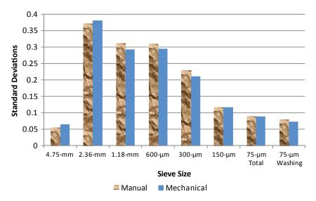
**Figure 4-3** Repeatability standard deviations of percent passing various sieve sizes after manual and mechanical washing pooled from AGF 171-172, AGF 175-176, and AGF 179-180 samples.
