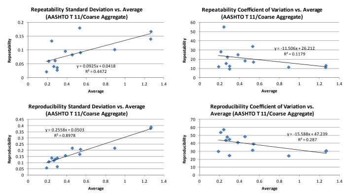
**Figure 3-3** Relationship between average and standard deviation and between average and coefficient of variation of percent material finer than a 75-µm (No. 200) sieve by washing of AGC.
