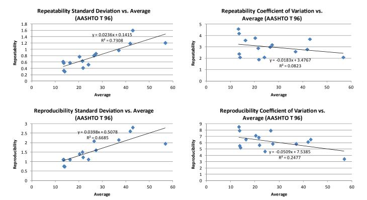
**Figure 3-1** Relationship between average and standard deviation and between average and coefficient of variation of the AASHTO T 96 test results.
