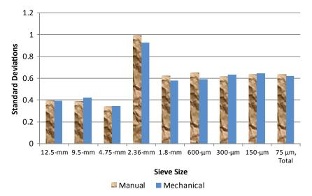
**Figure 4-8** Reproducibility standard deviations of percent passing various sieve sizes after manual and mechanical washing, pooled from HMASE 73-74, 75-76, and 77-78 samples.
