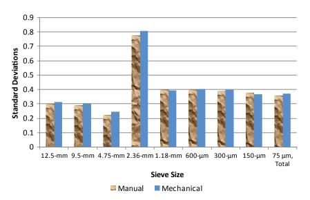
**Figure 4-7** Repeatability standard deviations of percent passing various sieve sizes after manual and mechanical washing pooled from HMASE 73-74, 75-76, and 77-78 samples.
