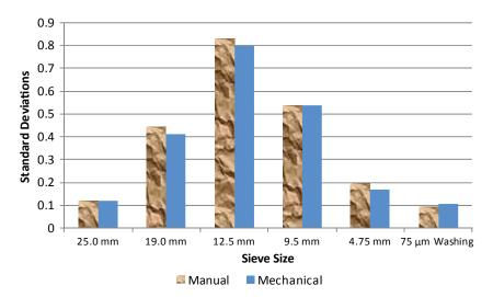
**Figure 4-1** Repeatability standard deviations of percent passing various sieve sizes after manual and mechanical washing pooled from AGC 169-170, AGC 173-174, and AGC 177-178 samples.
