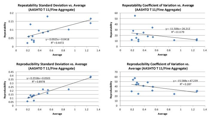
**Figure 3-4** Relationship between average and standard deviation and between average and coefficient of variation of percent material finer than a 75-µm (No. 200) sieve by washing of AGF.
