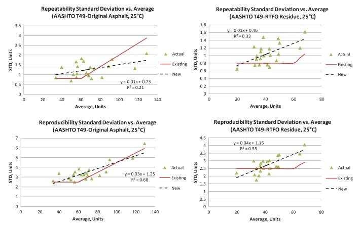
**Figure 2-10** Comparison of the existing and new repeatability and reproducibility standard deviations for penetration (AASHTO T 49) of original binder and RTFO residue at 25°C.
