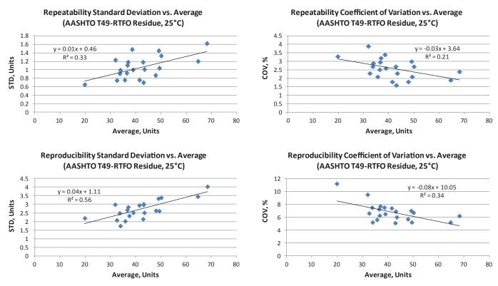
**Figure 2-8** Relationship between average and standard deviation and between average and coefficient of variation for penetration (AASHTO T 49) of RTFO residue at 25°C.
