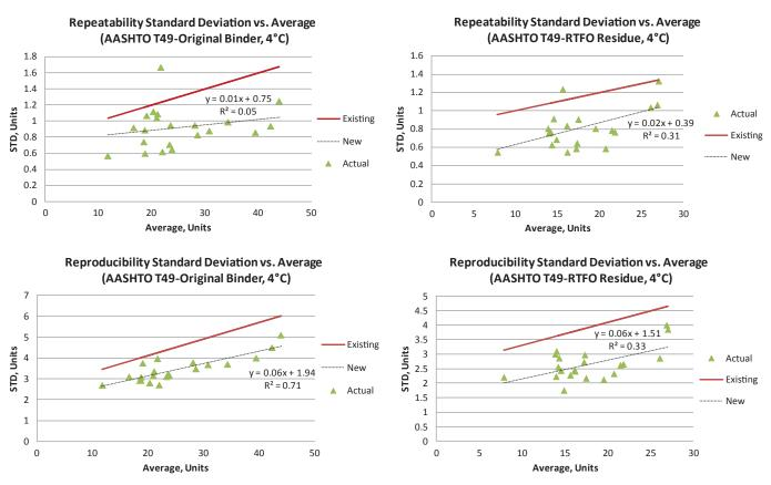
**Figure 2-9** Comparison of the existing and new repeatability/reproducibility standard deviations for penetration (AASHTO T 49) of original binder and RTFO residue at 4°C.
