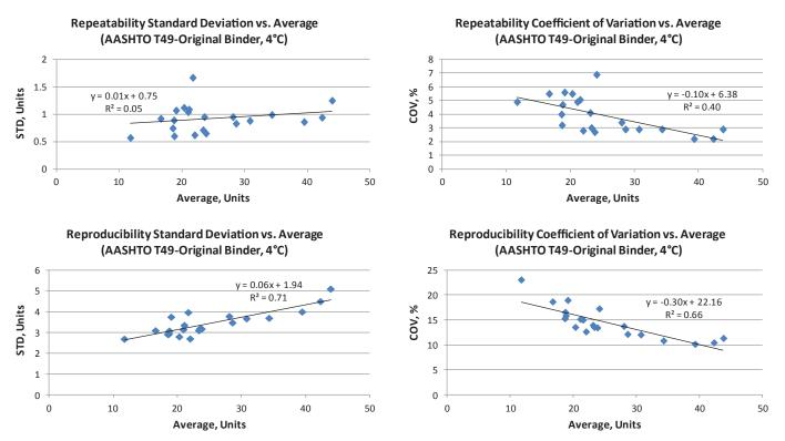
**Figure 2-5** Relationship between average and standard deviation and between average and coefficient of variation for penetration (AASHTO T 49) of original asphalts at 4°C.
