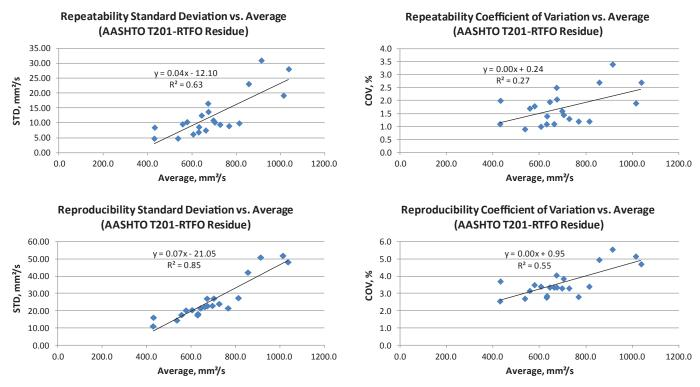
**Figure 2-2** Relationship between average and standard deviation and between average and coefficient of variation of kinematic viscosity (AASHTO T 201) test results for RTFO residue.
