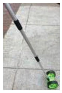
Figure 5-5. Measuring wheel.
