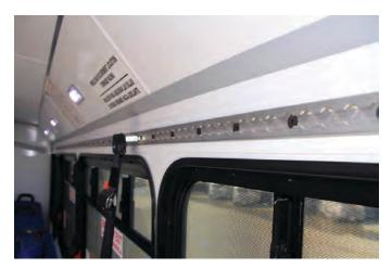
Figure 4-3. Continuous track for anchoring passenger shoulder strap, UTA FLEX bus vehicles (photo courtesy of TranSystems).
