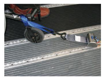
Figure 4-5. Tether strap attached to a wheelchair to assist with securement (photo courtesy of TranSystems).
