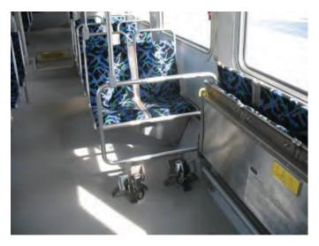
Figure 4-4. Modified "reach-through" panel behind securement area, designed by GET (photo courtesy of GET).
