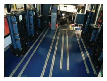
*Figure 4-1.* Laketran vehicle with full-length securement tracking, looking forward from the rear (photo courtesy of Laketran).
