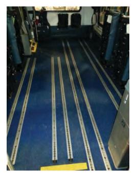
*Figure 4-2. Laketran vehicle with full-length securement tracking, looking rearward from the front. (photo courtesy of Laketran).*
