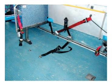
Figure 4-6. Supplemental strap used by LTD to secure scooters on fixed-route transit vehicles (photo courtesy of TranSystems).
