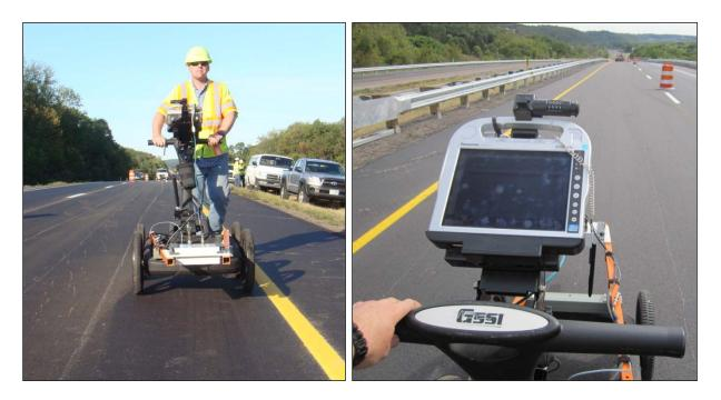
Figure 3.19. Collection of GPR data on SR-220 with real-time data processing.
