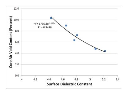
Figure B.1. Example calibration for calculating air voids.
