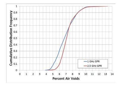
Figure 3.21. Expected distribution of air voids on SR-220.
