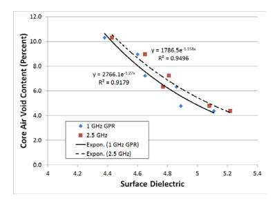
Figure 3.20. Calibration of air voids to GPR from SR-220.
