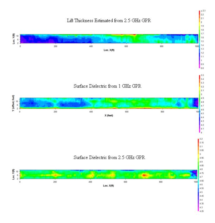
Figure 3.22. Lift thickness and surface dielectrics from SR-220.
