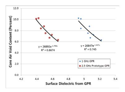
Figure 3.4. Calibration of air voids to GPR from US-29.
