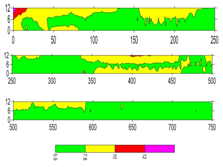
Figure 3.14. Geospatial distribution of air voids on Route 3 from 1 GHz GPR.
