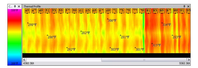
Figure 3.17. Excerpt of thermal profile for SP 6.33 placed 09/06/2013 on SR-220.
