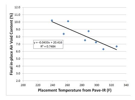
Figure 3.3. Relationship between air voids and placement temperature from US-29.
