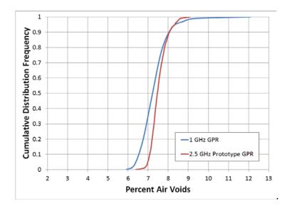
Figure 3.13. Expected distribution of air voids on Route 3 from GPR. Note: VDOT desired density is ≤7.8% air voids.
