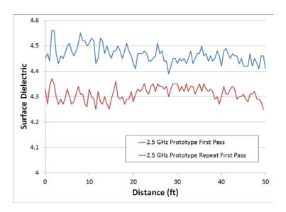
Figure 3.6. Shift in 2.5 GHz results during US-29 testing.
