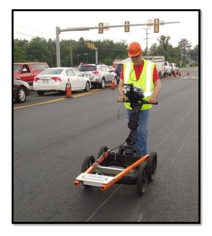
Figure ES.2. GPR System for measuring asphalt mixture uniformity.
