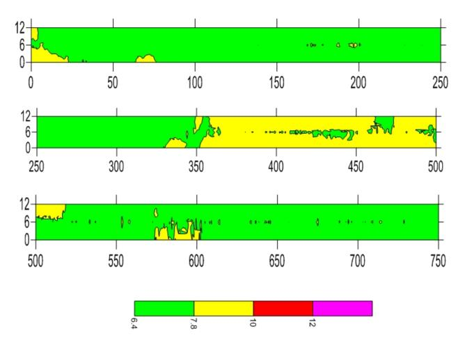
Figure 3.15. Geospatial distribution of air voids on Route 3 from 2.5 GHz GPR.
