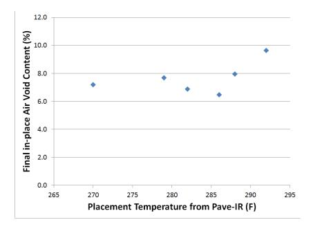
Figure 3.11. Scatter plot of air voids versus placement temperature from Route 3.
