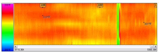
Figure 3.18. Thermal profile from last 1,000 ft of SR-220 placed 09/06/2013.
