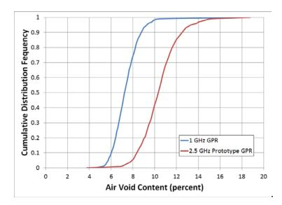
Figure 3.5. Expected distribution of air voids on US-29 from GPR. Note: VDOT desired density is  $\leq 7.8\%$  air voids.
