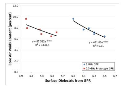
Figure 3.12. Calibration of air voids to GPR from Route 3.
