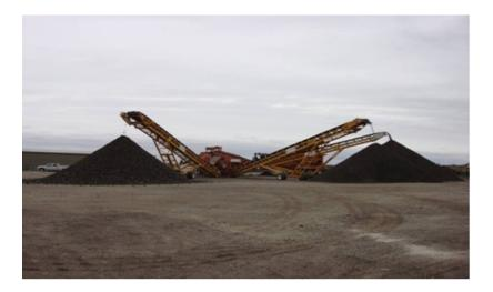
Figure B.3. PSI Technologies' state-of-the-art impact crushing and recycling of asphaltic rubble material.
