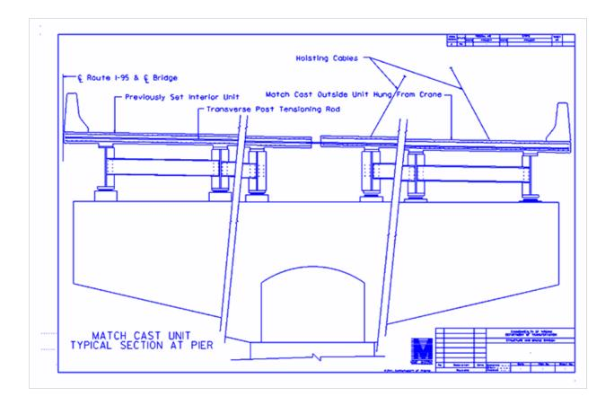
Figure B.32. Contractor-proposed change to bridge to use two sections (3).
