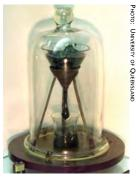
Bitumen can be extremely viscous and must be combined with lighter oils to move through pipelines. An experiment testing the viscosity of pitch at the University of Queensland, Australia, was begun in 1927; to date, only eight drops have fallen out of the funnel.
