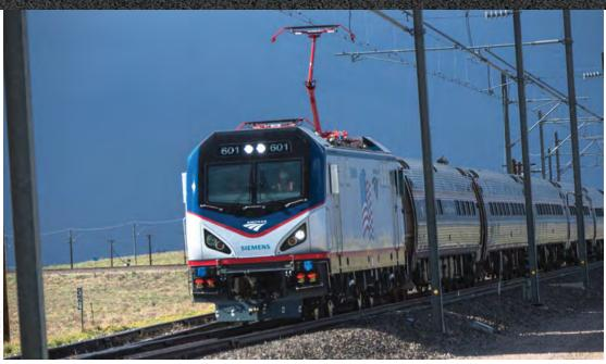
The new Amtrak Cities Sprinter high-speed electric locomotive undergoes tests at the U.S. DOT Transportation Technology Center in Pueblo, Colorado, in 2013.
