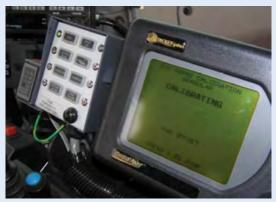
A ground-speed controller in calibration mode.
