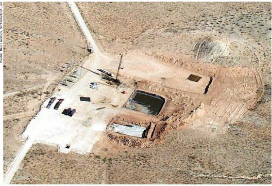
Drilling activity in the Permian Basin, which accounts for most of Texas' oil production. Roads at each site must be able to handle approximately 1,054 two-way truck trips.
