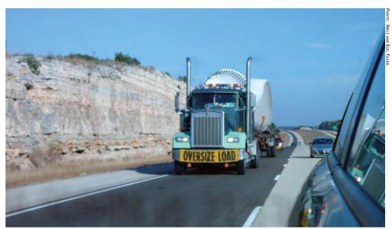
Trucks transporting wind turbine blades and other wind turbine components, mostly on Interstate highways, must obtain oversize and overweight permits.
