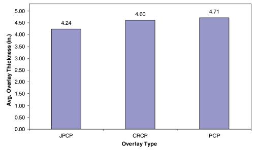
Figure B.36. Average overlay thickness for SPS-7 overlay types.
