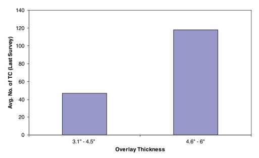
Figure B.40. JPCP overlay thickness versus number of transverse cracks.
