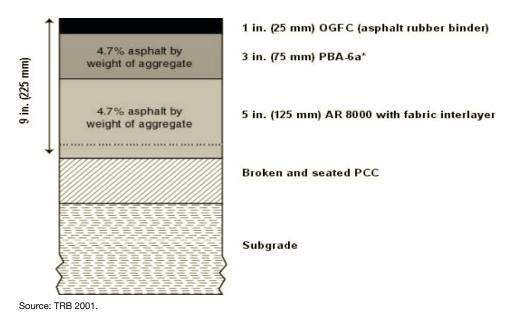
Figure A.7. Cross-sectional design for the I-710 Freeway.
