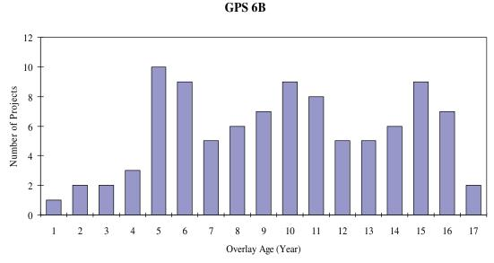
Figure B.2. Frequency of overlay age within experiment GPS-6B.
