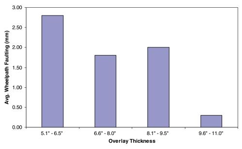
Figure B.26. Overlay thickness versus average wheelpath faulting.
