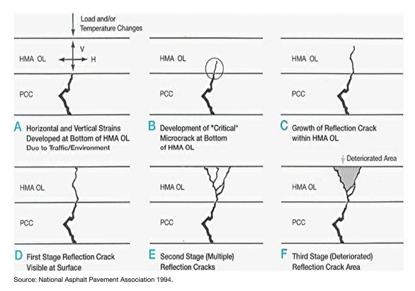
Figure A.14. Growth of a reflection crack.
