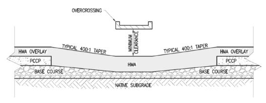
Figure 3.8. Illustration of flexible pavement transitions to overcrossings.
