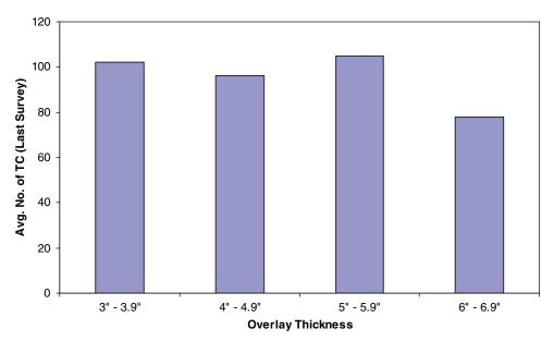
Figure B.42. CRCP and PCP overlay thickness versus number of transverse cracks.
