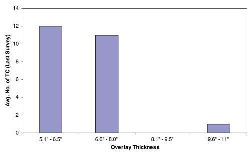
Figure B.16. JPCP overlay thickness versus average number of transverse cracks.
