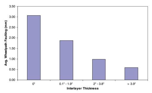
Figure B.29. JPCP interlayer thickness versus average wheelpath faulting.
