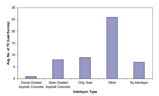
Figure B.27. JPCP interlayer type versus average number of transverse cracks.
