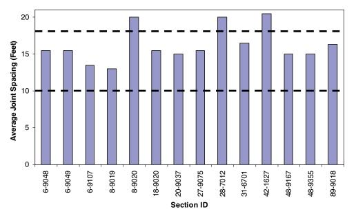
Figure B.13. JPCP average joint spacing.
