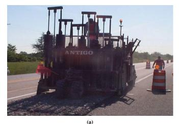
Figure A.9. (a) Multihead breaker. (b) Grid roller.
