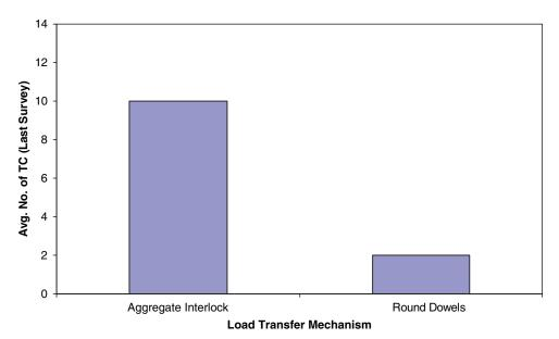
*Figure B.32. JPCP load-transfer mechanism versus average number of transverse cracks.*
