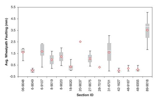
Figure B.25. Distribution of average wheelpath faulting by section.
