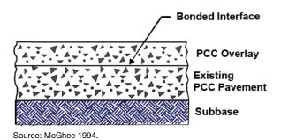
Figure A.25. Typical cross section of a bonded PCC overlay.
