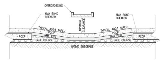
Figure 3.9. Illustration of rigid pavement transitions to overcrossings.
