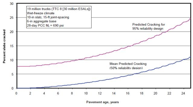
Figure D.1. Slab cracking.
