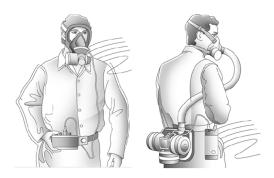
**FIGURE 2-1** Examples of tight-fitting powered air purifying respirators. SOURCE: OSHA, 2011.
