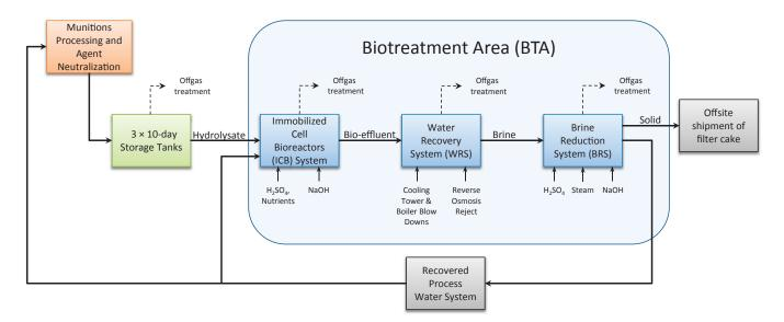
FIGURE 7-1 PCAPP BTA process diagram. SOURCE: Adapted from Don Guzzetti, start-up field supervisor, PCAPP, and Dave deLesdernier, support, Battelle, "Biotreatment Area Risk Reduction and Mitigation," presentation to the committee on July 29, 2014.
