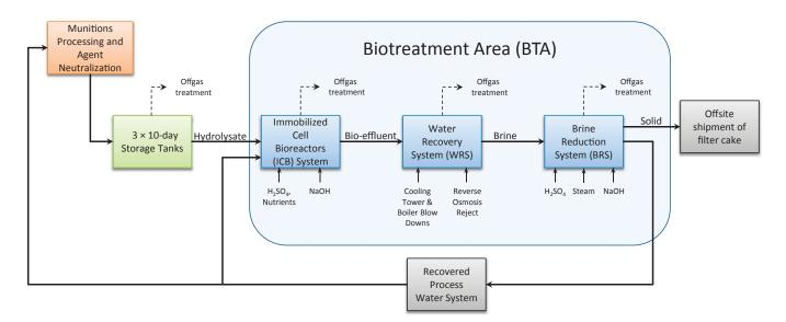
FIGURE 2-1 PCAPP biotreatment area process diagram. SOURCE: Adapted from Don Guzzetti, start-up field supervisor, PCAPP, and Dave DeLesdernier, support, Battelle, "Biotreatment Area Risk Reduction & Mitigation," presentation to the committee on July 29, 2014.
