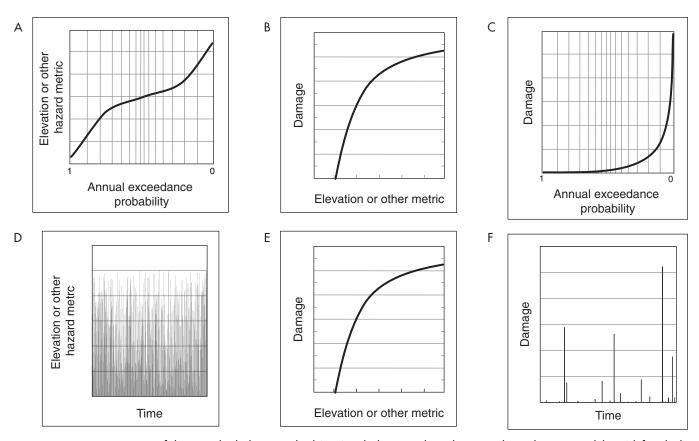
**FIGURE 3.8** Comparison of the NFIP hydrologic method (a–c) with the event-based approach used in cat modeling (d–f), which creates a long history of flood events, then estimates and averages the damage associated with each to compute average annual loss. SOURCE: Courtesy of David Ford, David Ford Consulting Engineers, Inc.
