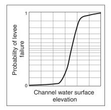
**FIGURE 3.4** Variability in the performance of flood protection systems, such as levees, is represented with a fragility function, which is included in the risk assessment. SOURCE: Courtesy of David Ford, David Ford Consulting Engineers, Inc.
