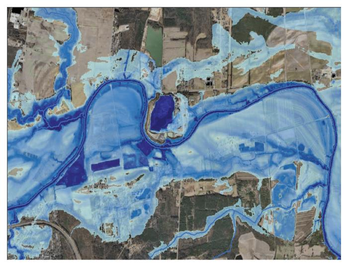
**FIGURE 3.9** One percent annual chance exceedance depth grid along a reach of the Tar River in Rocky Mount, North Carolina. Darker blues represent greater flood depth between the base flood elevation and the terrain elevation. SOURCE: Courtesy of John Dorman, North Carolina Floodplain Mapping Program.
