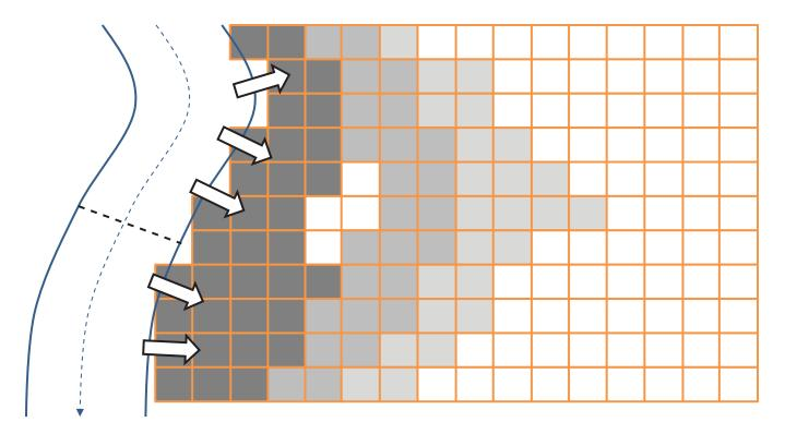
**FIGURE 3.3** For complex floodplains, water surface elevations on the floodplain may be computed with a two-dimensional model. SOURCE: Courtesy of David Ford, David Ford Consulting Engineers, Inc.
