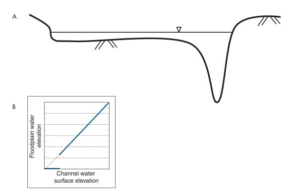
**FIGURE 3.2** Water surface elevations on the floodplain adjacent to a river may be inferred from the elevation at a cross section of the river using a floodplain-channel water surface elevation function. (a) A cross section of the river and adjacent floodplain. In (b), the floodplain depth is zero until the capacity of the channel is exceeded and water moves onto the floodplain. SOURCE: Courtesy of David Ford, David Ford Consulting Engineers, Inc.
