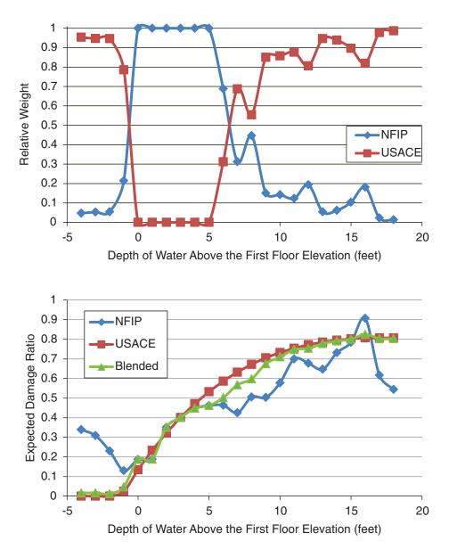
**FIGURE 4.5** Illustration of the NFIP credibility analysis for 2005 loss data. (Top) Relative weights assigned to the NFIP data and the USACE data based on the credibility weighting methodology. (Bottom) Comparison of the NFIP claims data, USACE damage estimates, and the blended result using the credibility weighting methodology.
