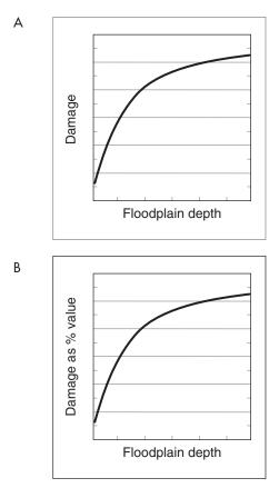
**FIGURE 3.5** Exposure and vulnerability are represented with an inundation depth-damage function (a), which may be developed from a generic inundation depth-percent damage function, scaled by the total value of the asset (b). SOURCE: Courtesy of David Ford, David Ford Consulting Engineers, Inc.
