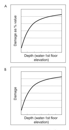
**FIGURE 3.7** NFIP DELV curves predict damage as a function of depth of water relative to the lowest floor elevation of the structure. SOURCE: Courtesy of David Ford, David Ford Consulting Engineers, Inc.
