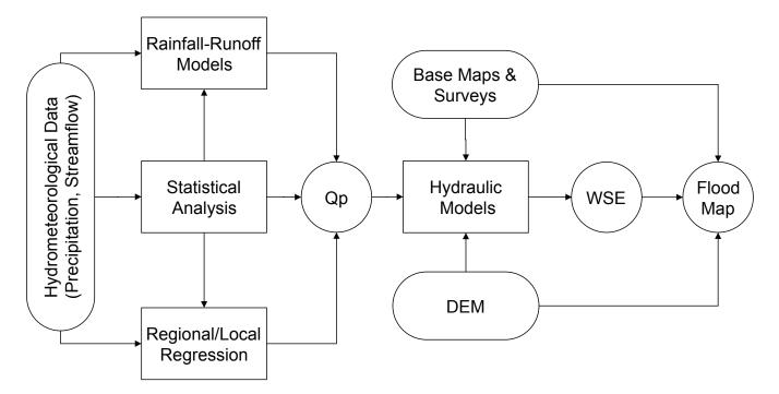
**FIGURE 2.1** Schematic of an idealized riverine flood study showing the data inputs (rounded boxes), models and methods used in the hydrologic and hydraulic analysis (boxes), and outputs (circles), including the flood discharge (Qp) and the water surface elevation (WSE). Note: DEM = digital elevation model. SOURCE: NRC (2009).
