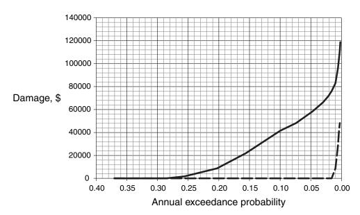
FIGURE 4.1 Illustration of a damage-exceedance probability function for the same structure at two elevations. (Solid line) Lowest floor elevation 4 feet below the base flood elevation (negatively elevated structure). (Dashed line) Lowest floor elevation equal to the base flood elevation.
