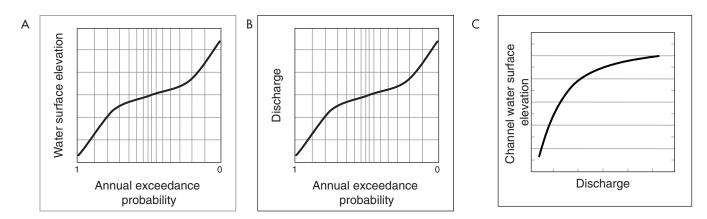
**FIGURE 3.1** (a) Flood hazard for riverine systems may be represented with a water surface elevation–exceedance probability function, usually derived from flood studies. Alternatively, the function may be derived from a discharge–exceedance probability function (b), transformed with a discharge–water surface elevation function (c). The annual exceedance probability means the same thing as the annual chance of exceedance. SOURCE: Courtesy of David Ford, David Ford Consulting Engineers, Inc.
