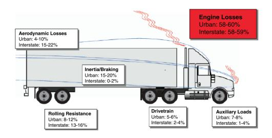
FIGURE 5-1 Energy "loss" range of vehicle attributes as impacted by duty cycle, on a level road. SOURCE: NRC (2010), Figure 5-8.
