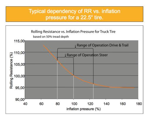
**FIGURE 5-3** Typical dependency of rolling resistance on inflation pressure for a 22.5 in. tire. SOURCE: J. Kleffmann, Continental, "Effect of Tire Inflation on Rolling Resistance," Presentation to NRC Committee on Assessment of Technologies and Approaches for Reducing the Fuel Consumption of Medium- and Heavy-Duty Vehicles, Phase 2, November 21, 2013.
