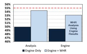
FIGURE 3-2 Cummins-Peterbilt SuperTruck team's analysis and results using AFCI at 1,000 rpm and 10 bar. SOURCE: L. Kocher, "SuperTruck 55% BTE Update Technology and System Level Demonstration of Highly Efficient and Clean, Diesel Powered Class 8 Trucks," presentation to the committee, Columbus, Indiana, August 28, 2014, slide 24. SuperTruck Annual Merit Review Presentations, Cummins, Inc.
