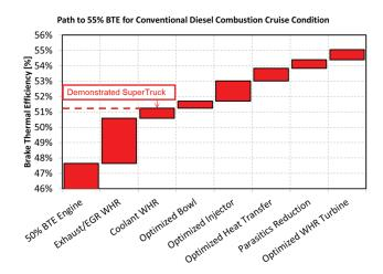
FIGURE 3-1 Cummins-Peterbilt SuperTruck team's projected incremental gains to get from its current 50 percent BTE engine to 55 percent BTE. SOURCE: L. Kocher, "SuperTruck 55% BTE Update Technology and System Level Demonstration of Highly Efficient and Clean, Diesel Powered Class 8 Trucks," presentation to the committee, Columbus, Indiana, August 28, 2014, slide 20. SuperTruck Annual Merit Review Presentations, Cummins, Inc.
