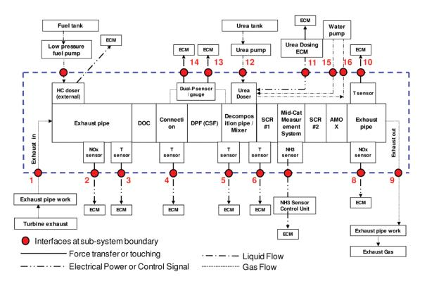
**FIGURE 3-7** Example of OBD layout for a 2013 HD aftertreatment system. SOURCE: D. Stanton, "Systematic Development of Highly Efficient and Clean Engines to Meet Future Commercial Vehicle GHG Regulations," *SAE Int. J. Engines* 6(3): 1395-1480. Reprinted with permission from SAE paper 2013-01-2421 Copyright © 2013 SAE International.
