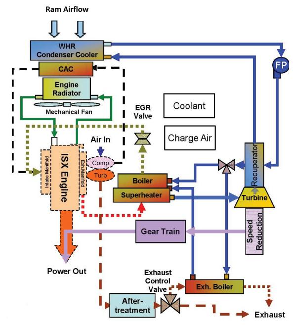
FIGURE 8-1 Cummins Demonstrator 1 WHR system layout. SOURCE: Koeberlein (2014).
