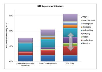
**FIGURE 3-4** Volvo SuperTruck team's stack chart of the incremental improvements in engine technology to reach 55 percent BTE from a concept demonstration powertrain. SOURCE: A. Greszler, "SuperTruck Development and Demonstration of a Fuel-Efficient Class 8 Highway Vehicle," presentation to the committee, May 14, 2014, slide 14. Volvo Group Truck Technology.
