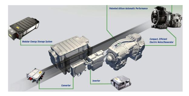
FIGURE 4-2 Allison H 3000 hybrid transmission major components. SOURCE: Allison (2015). © Allison Transmission 2011. All rights reserved.
