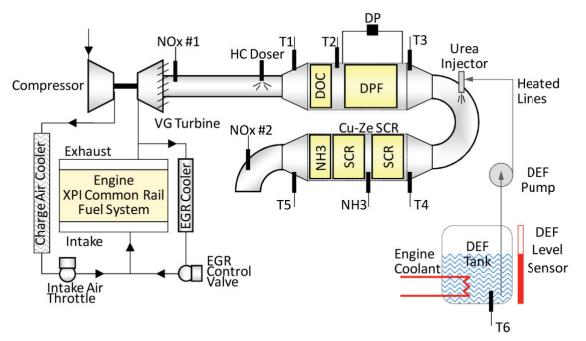
**FIGURE 3-6** Layout of a modern HD diesel emission control system. SOURCE: D. Stanton, "Systematic Development of Highly Efficient and Clean Engines to Meet Future Commercial Vehicle GHG Regulations," *SAE Int. J. Engines* 6(3): 1395-1480. Reprinted with permission from SAE paper 2013-01-2421Copyright © 2013 SAE International.
