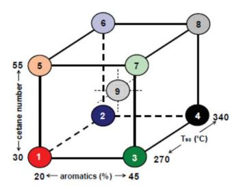
**FIGURE 3-8** Fuels for advanced combustion engines (FACE) diesel fuel set. SOURCE: B. Zigler, "Fuels for Advanced Combustion Engines," DOE Annual Merit Review FJ002, May 15, 2012. National Renewable Energy Laboratory.
