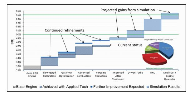
**FIGURE 3-5** Navistar SuperTruck team's projected improvements in the engine technologies that will enable them to achieve 55 percent BTE. SOURCE: R. Nine and R. Zukouski, "SuperTruck–Development and Demonstration of a Fuel-Efficient Class 8 Tractor & Trailer Vehicle System," presentation to the committee, November 18, 2014, slide 12.
