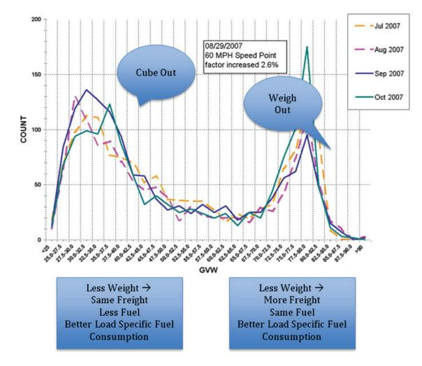
**FIGURE 5-4** Bimodal distribution of truck gross vehicle weight (GVW) for five-axle vehicles from Weigh-In-Motion (WIM) data 421. SOURCE: Quinley (2010).
