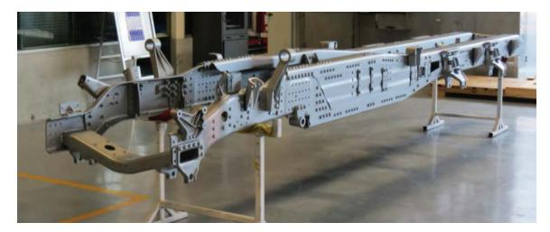
FIGURE 8-3 Prototype Volvo aluminum tractor frame. SOURCE: Amar (2014).
