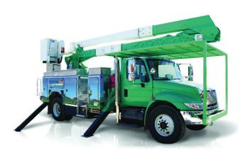
**FIGURE 4-1** Odyne Class 6 plug-in hybrid utility lift truck. SOURCE: Green Fleet Magazine (2008). Courtesy of Odyne Systems, LLC.
