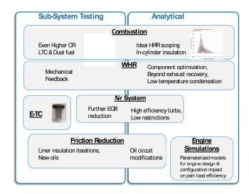
**FIGURE 3-3** Overview of Daimler SuperTruck team's approach to achieving 55 percent BTE. SOURCE: Singh (2014). NOTE: E-TC, electronic turbocharger; CR, combustion ratio; LTC, lowtemperature combustion; HRR, heat release rate; WHR, waste heat recovery; EGR, exhaust gas recirculation.
