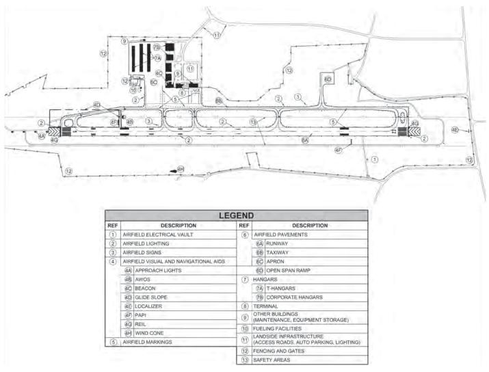
*Figure 3.1.* Airport infrastructure systems. Source: Delta Airport Consultants, Inc. Notes: AWOS = automated weather observing systems, PAPI = precision approach path indicator, REIL = runway-end identifier light.
