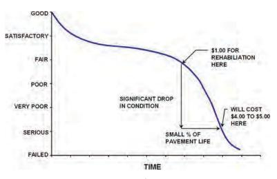
*Figure 4.1. Typical pavement life cycle. Source: FAA Central Region, Guidance—Airport Obligations: Pavement Maintenance.*
