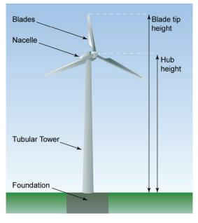
*Figure 1-10.* Components of a utility-scale wind turbine.
