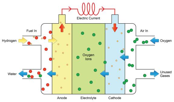
Figure 1-16. Schematic of a fuel cell.
