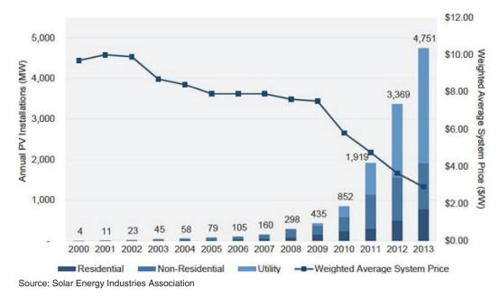
Figure 1-4. Solar installations and system price over time.
