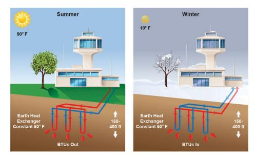
Figure 1-7. Schematic of geothermal heat pump.
