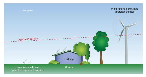
*Figure 2-16. Examples of structures that may impinge on airspace.*
