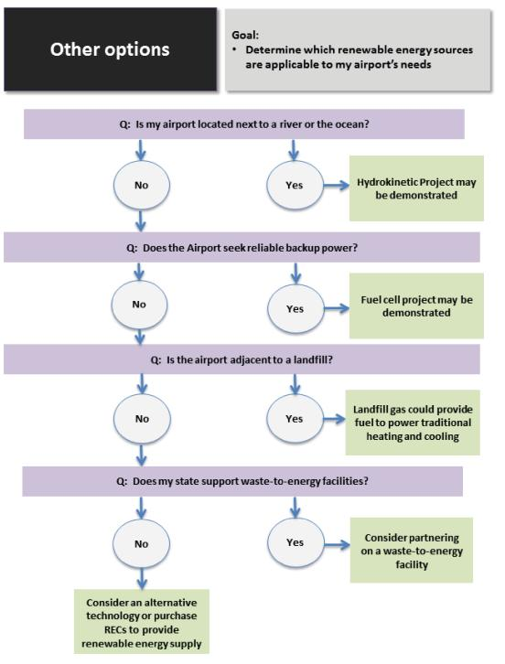
Figure 2-24. Other technologies process flow chart.
