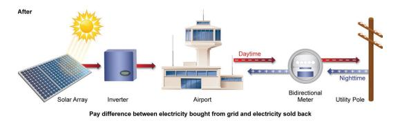
E Excess energy not used by airport that goes back to the grid E Energy used by airport from the grid
