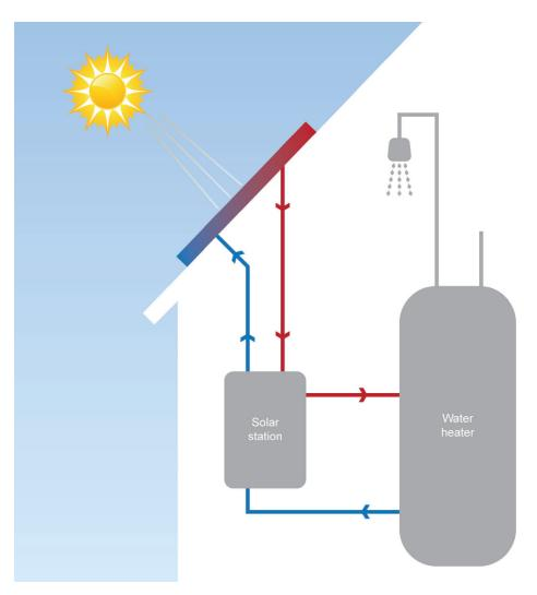
Figure 1-6. Schematic of a solar thermal system.
