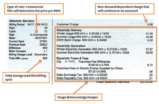
Figure 1-18. Utility bill example showing different rates and charges.
