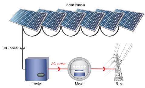
Figure 1-3. Schematic of a solar photovoltaic string.
