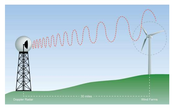
Figure 2-18. Wind turbines as physical obstructions to radar signals.
