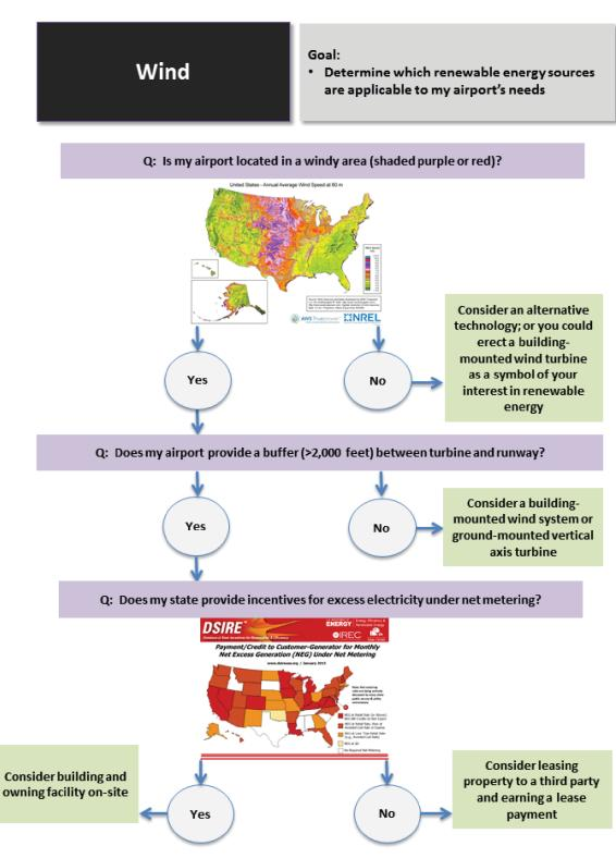
Figure 2-21. Wind process flow chart.
