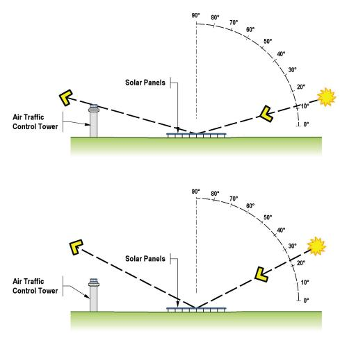
*Figure 2-17.* Illustration of geometric factors associated with glare on sensitive receptors.
