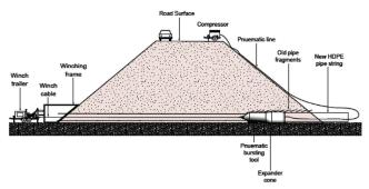
FIGURE 34 Pipe bursting schematic (USDA Forest Service 2005).
