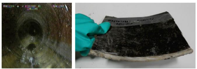
FIGURE 33 Video inspection of CIPP liner after 23 years of service (*left*) and cut section of liner after 34 years of service (*right*) confirming excellent performance and no measurable deterioration (Macey and Zurek 2012).
