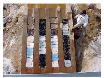
FIGURE 9 Caltrans abrasion test panel installation showing various culvert materials and coatings (Caltrans 2013).
