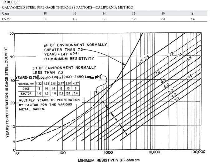
FIGURE B2 Chart for estimating years to perforation of steel culverts using California method (Caltrans 1999).
