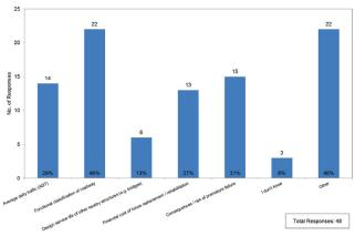
FIGURE 3 Agency bases for determining the design service life of culverts.
