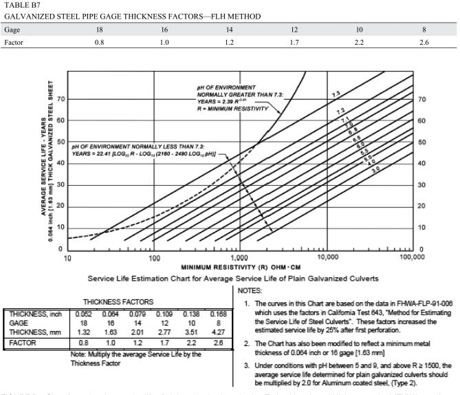
FIGURE B4 Chart for estimating service life of plain galvanized steel using Federal Lands and Highway method (FHWA 2008).
