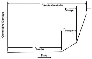
FIGURE 20 Steel-reinforced concrete corrosion service life diagram (FDOT 2014b).
