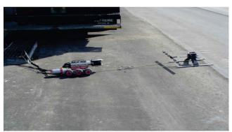
FIGURE 35 Laser profiler and CCTV used in tandem for pipe inspections.
