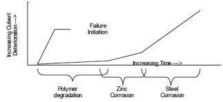
FIGURE 24 Polymer-coated CSP service life model (Ault 2003).
