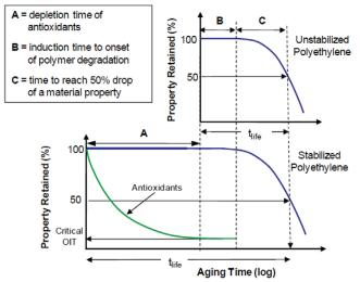
FIGURE 11 Schematic of time-dependent oxidation degradation mechanism for polyethylene (M. Paredes, FDOT, personal communication, May 5, 2014).
