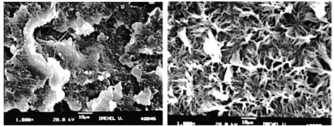
FIGURE 12 Microscope images of HDPE crack surfaces (Hsuan and McGrath 1999): (*left*) flake morphology characteristic of impact-type fracture; (*right*) fibrous morphology characteristic of slow crack growth.
