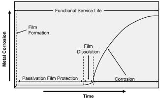
FIGURE 7 Life-cycle schematic of metal corrosion (after M. Paredes, FDOT, personal communication, May 5, 2014).
