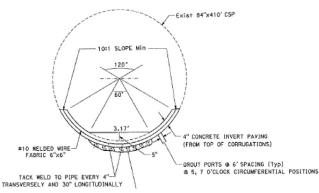
FIGURE 28 Standard detail for concrete invert paving (Caltrans 2013).
