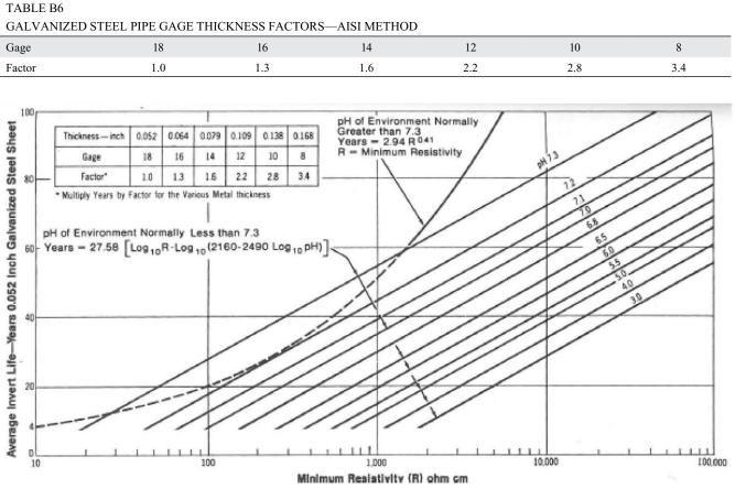
FIGURE B3 Chart for estimating average invert life using AISI method (AISI 1994).
