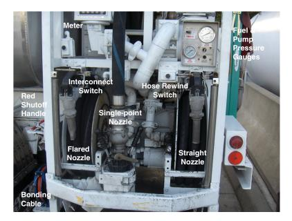
FIGURE 17 Different nozzles used on jet fuel truck dispenser. (*Courtesy*: S. Quilty, SMQ Airport Services.)
