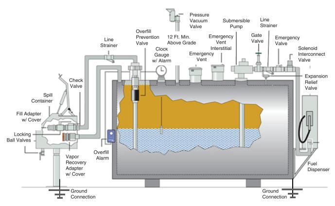
FIGURE 21 Components for a horizontal AST. (Adapted from Morrison Bros.) Used with permission.
