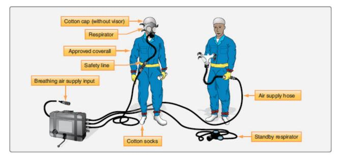
FIGURE 25 Equipment required for certified confined space fuel tank entry. (*Courtesy:* FAA Aviation Maintenance Technician Handbook—Airframe 2012.)
