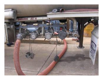
FIGURE 4 Example of a dedicated Jet A tanker delivering fuel to an airport tank farm. (*Courtesy*: S. Quilty, SMQ Airport Services.)
