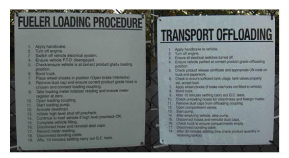
FIGURE 28 Example of procedures to load and offload fuel posted at transfer station. (*Courtesy*: S. Quilty, SMQ Airport Services.)
