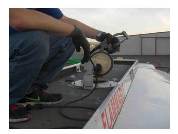
FIGURE 26 Example of employee monitoring mobile tank fill and operating an enabling switch. (*Courtesy:* S. Quilty, SMQ Airport Services.)
