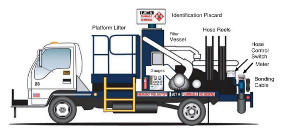
FIGURE 11 Example of a mobile platform lifter hydrant transfer vehicle. (*Courtesy*: A. Villaverde, LaxFuel Corporation.)
