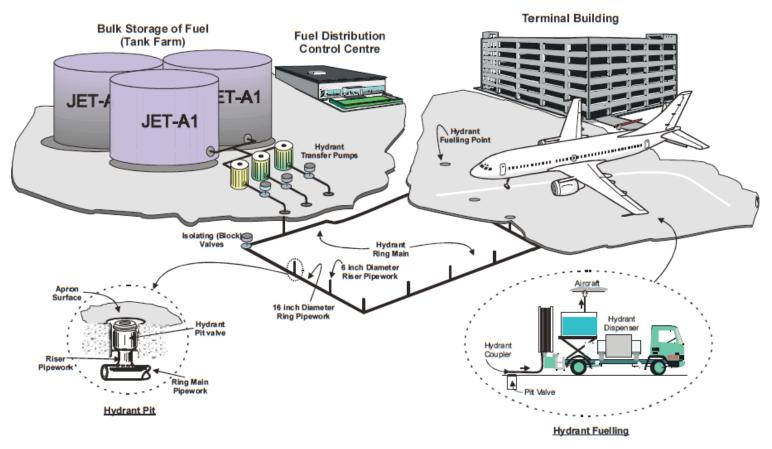
FIGURE 8 Typical fuel hydrant delivery system. (Courtesy: Jones et al. 2000, p. 15.)
