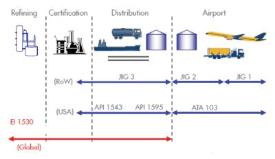
FIGURE 22 Comparison of API, ATA, JIG, and EI standards and point of industry application. RoW = rest of world. (*Courtesy*: Shell Aviation Limited.) Used with permission.
