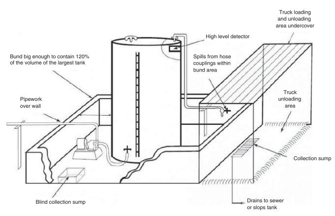
FIGURE 15 Typical aboveground tank with containment and spill protection. (Courtesy: Flexibund, Australia.) Used with permission.
