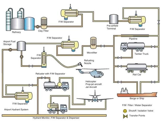
FIGURE 3 Fuel delivery diagram from refinery to aircraft showing filtration points and transportation modes. (*Courtesy*: FAUDI Aviation.) Used with permission.
