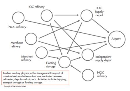
FIGURE 2 Schematic of various relationships for fuel delivery to an airport. NOC = national oil company; IOC = independent oil company. (*Courtesy*: Shell Oil Company.) Used with permission.
