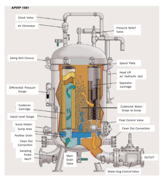
FIGURE 20 Typical fuel coalescer filter system for bulk storage. (Adapted from Precision Filtration Products.) Used with permission.
