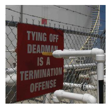
FIGURE 27 Sign designed to deter an unsafe fuel loading practice. (*Courtesy*: S. Quilty, SMQ Airport Services.)
