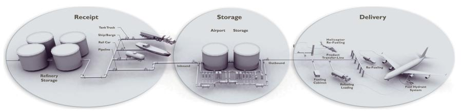
FIGURE 1 Fuel delivery system from refinery to aircraft. (Source: "Aviation Fueling: Technology Update." Courtesy: Hatch Mott MacDonald.) Used with permission.
