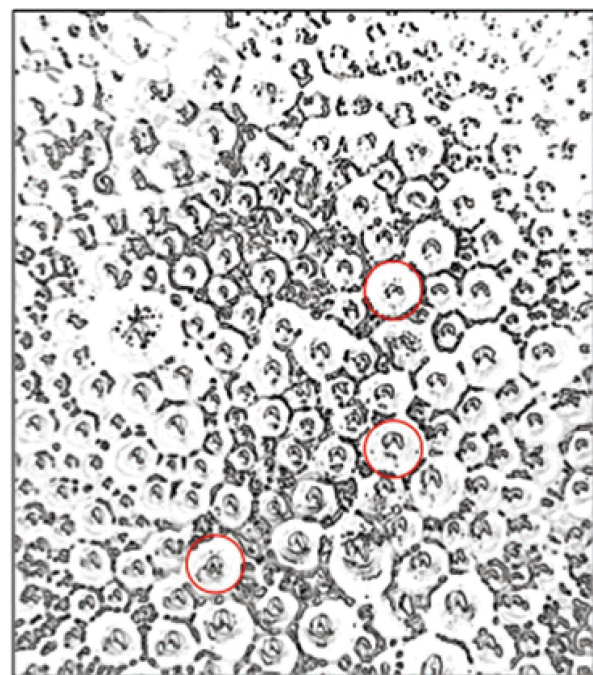
Figure 3-10. Surface of binder A6 at approximately 30 s after foaming in the Wirtgen foamer with 3.0% (left) and 1.0% (right) water content.
