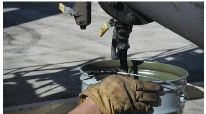
Figure 4-37. Free-flowing foamed binder sample, Huntsville, Texas.
