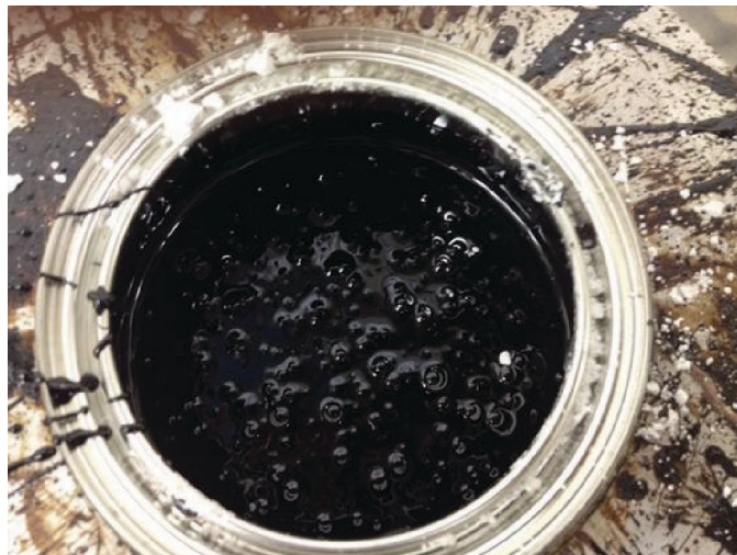
Figure 3-25. Bubble size of foam produced using zeolite.
