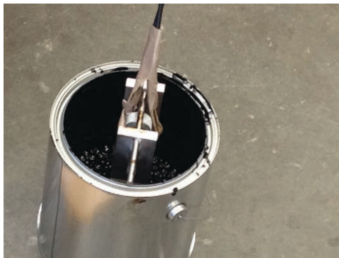
Figure 2-3. Ultrasonic density test setup.
