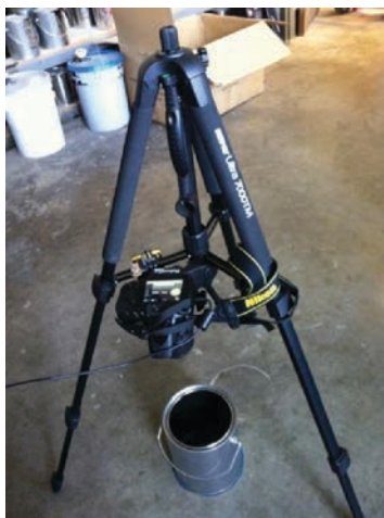
Figure 1. Camera setup for digital image capture of foamed binder sample.
