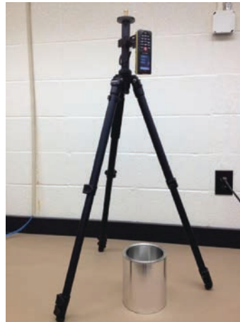
Figure 2. Illustration of the LDM pointing into an empty can for calibration.
