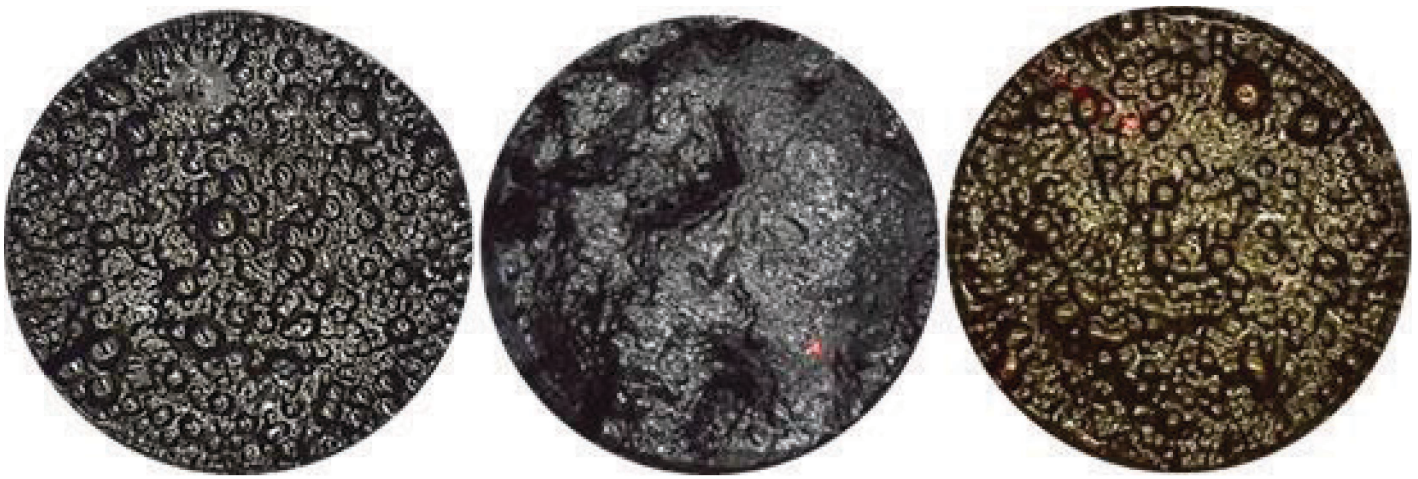
Figure 3-20. Surface of the foamed binder 5 s after foaming in the Wirtgen foamer: (a) without additive, (b) with additive F1, and (c) with additive W1.
