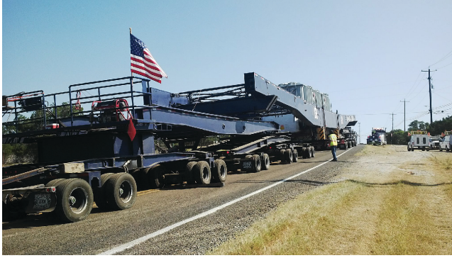
FIGURE 18 Vehicle of 1.2 million lb GVW traveling from Houston to Flat Rock, Texas.
