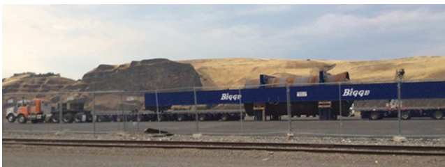
FIGURE 19 Vehicle of 792 kips GVW traveling from Eastern Washington to the Idaho Border.
