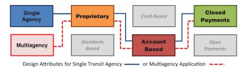
*Figure 4-3. Single or multiagency, proprietary, card-based, closed payment system design.*
