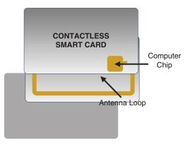
*Figure 5-3. Elements of a contactless smart card.*
