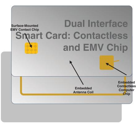
Figure 6-2. Dual-Interface Card (Contactless & EMV Chip).
