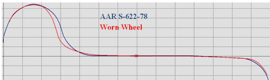
Figure 3. Existing Wheel Template and Worn Wheel Profiles
