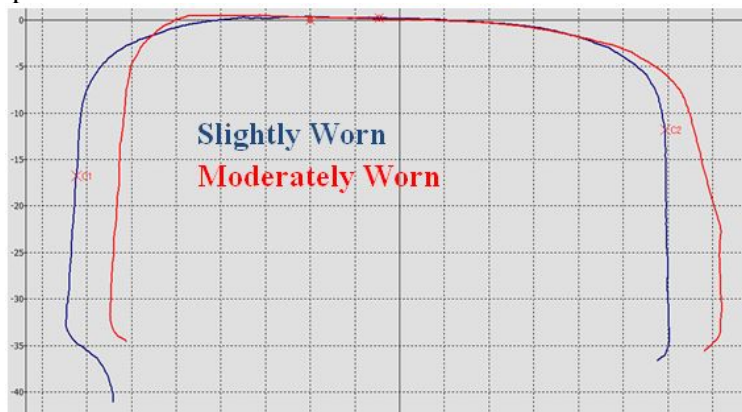
Figure 24. Slightly Worn and Moderately Worn Rail Profiles Measured on Tangent Track
