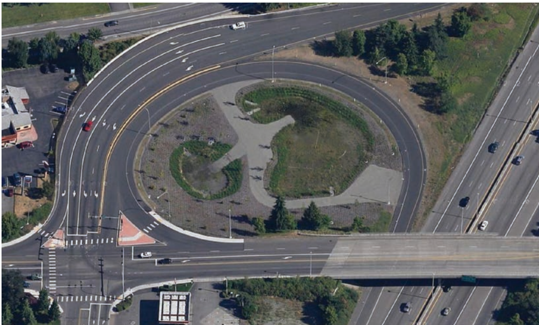
Figure 20. Example of project drainage and grading configuration developed to use available space at interchange, Tumwater, WA. Source: Google Earth Professional.
