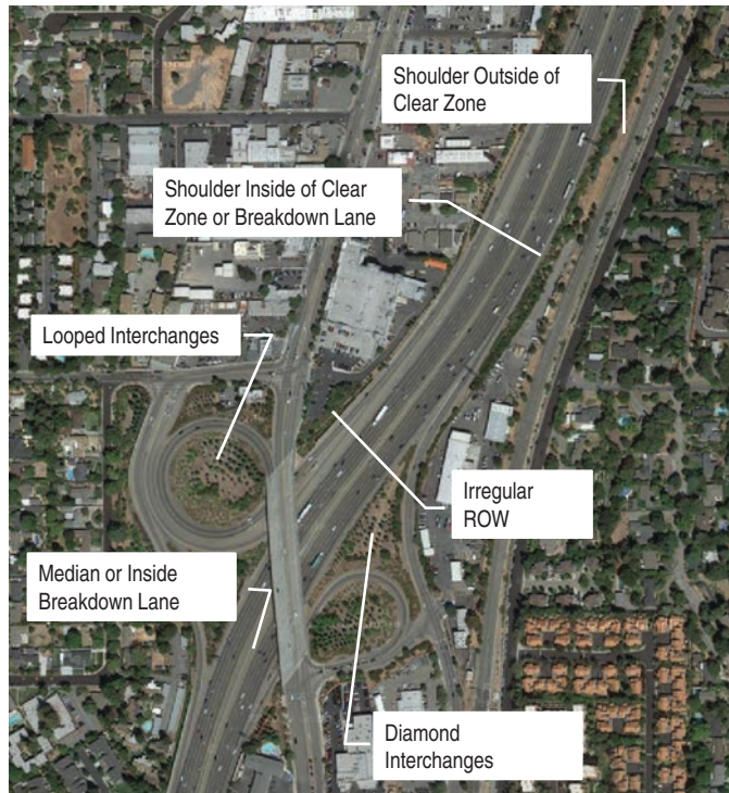
Figure 23. Key to common geometric opportunities within urban highway environments (hypothetical opportunities shown).
