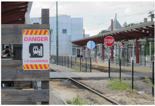
Figure 30. Example of a stop sign used between tracks to indicate train operators should stop train prior to the pedestrian-rail crossing.
