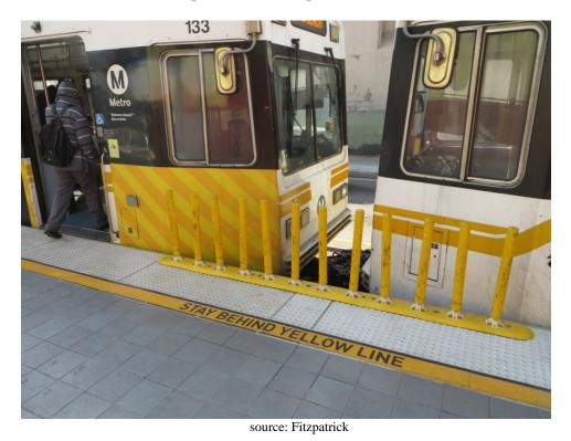
Figure 96. Flexible delineators between ends of rail cars prevent visually impaired travelers from falling between cars.
