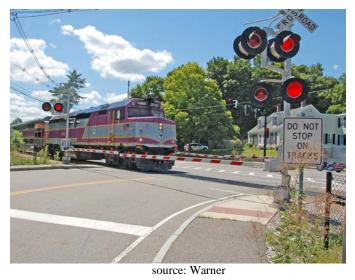
Figure 32. Example of single automatic gate for both sidewalk and roadway.
