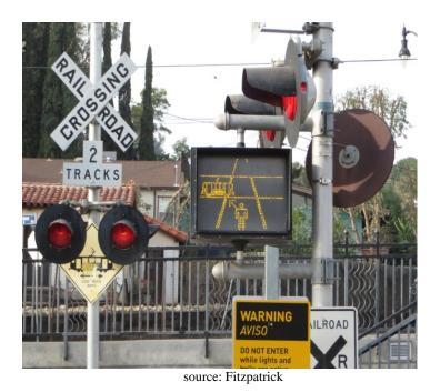
Figure 91. The pictogram within this blank out sign shows a side view of a train approaching from the left.
