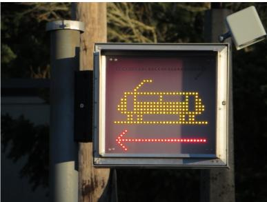
Figure 66. Example of active blank out signal with audible warning.
